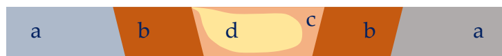
Figure 2. Typical cross section of a friction stir welded joint: (a) Unaffected material; (b) Heat-affected zone (HAZ); Thermomechanically affected zone (TMAZ); Weld nugget o Stirring zone (SZ).
