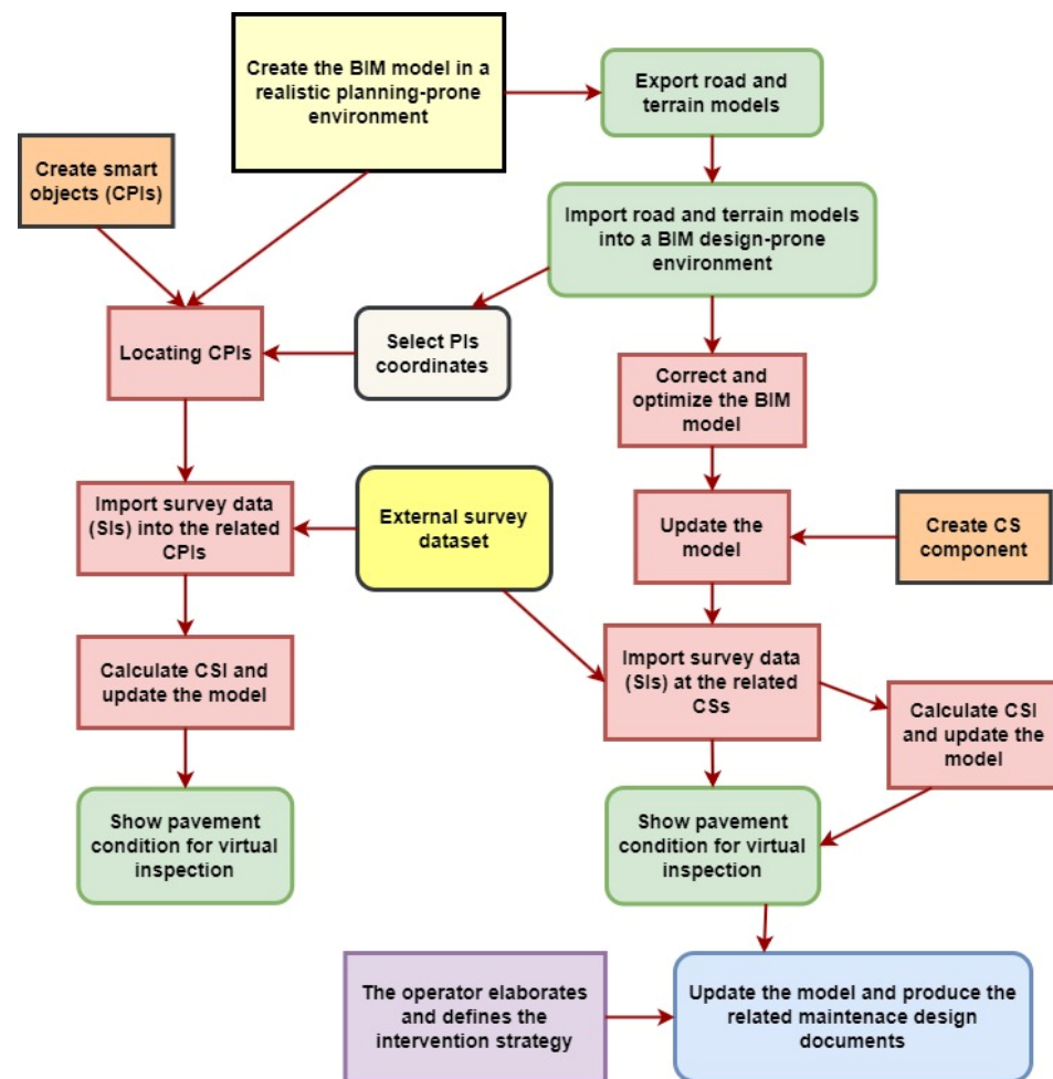
Figure 1. Flowchart of the proposed operative framework (CPI: Condition Point of Interest; PI: Point of Interest; CS: Condition Subassembly; SI: State Indicator; CSI: Critical State Index).
