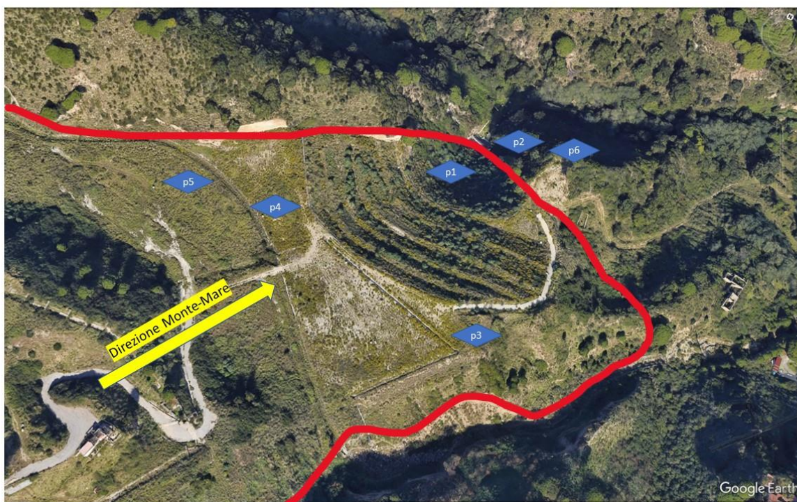
Figure 39: Image of the landfill with the location of the piezometers highlighted and the uphill-seaward direction. The landfill boundary is indicated in red.
