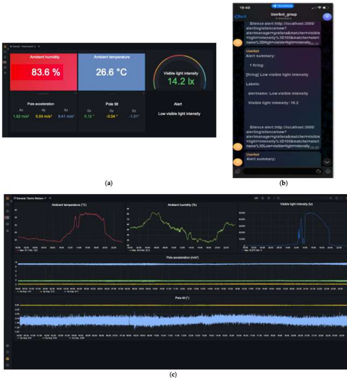
Figure 5.20: Typical interface, (a) indicators and (c) graphs customized by the users on Grafana for desktop terminals, and typical alert for smartphone on Telegram app (b).
