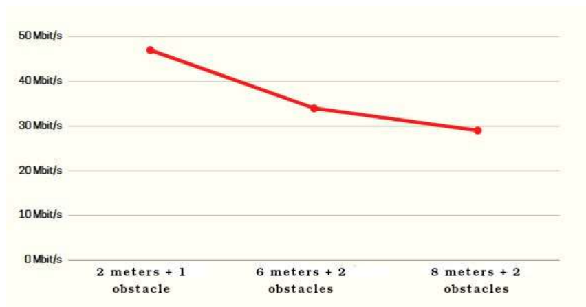
Figure 10.15: Transmission rate with obstacles.
