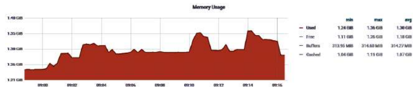
Figure 4.8: Memory usage request in case of flow of 500 get requests.
