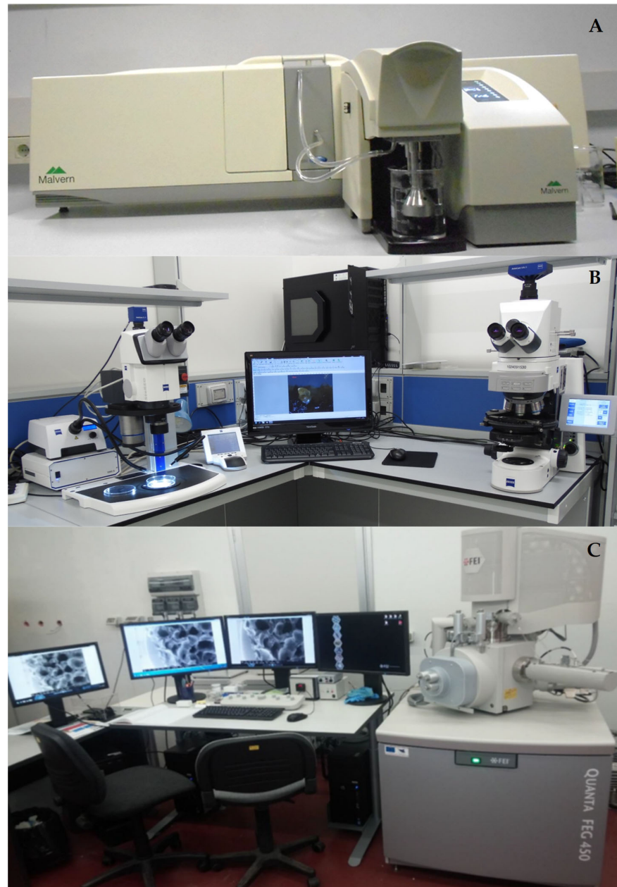
Figure 3. Instrumentation. (A) Laser diffraction granulometer. (B) Workstation—Motorized stereomicroscope with reflected and transmitted polarized light (on the left), motorized petrographic optical microscope with reflected and transmitted polarized light (on the right), and workstation (in the center)—Forensic Geology laboratory, MIFT Department, University of Messina. (C) SEM equipped with EDS system and workstation—Laboratory of microscopic analyses, Engineering Department, University of Messina. Source: Author.
