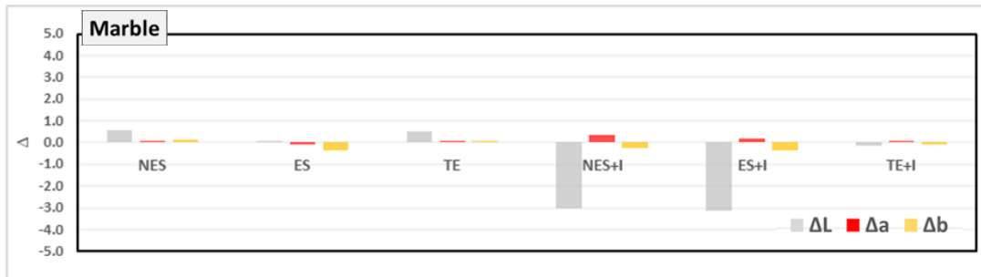
Figure 6. \Delta E value with its components ( \Delta L , \Delta a , \Delta b ) for each treatment on marble surfaces.
