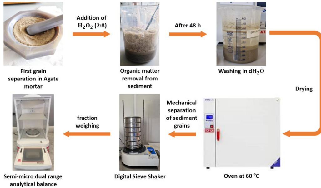
Figure 17. Sediment granulometry process schematization.
