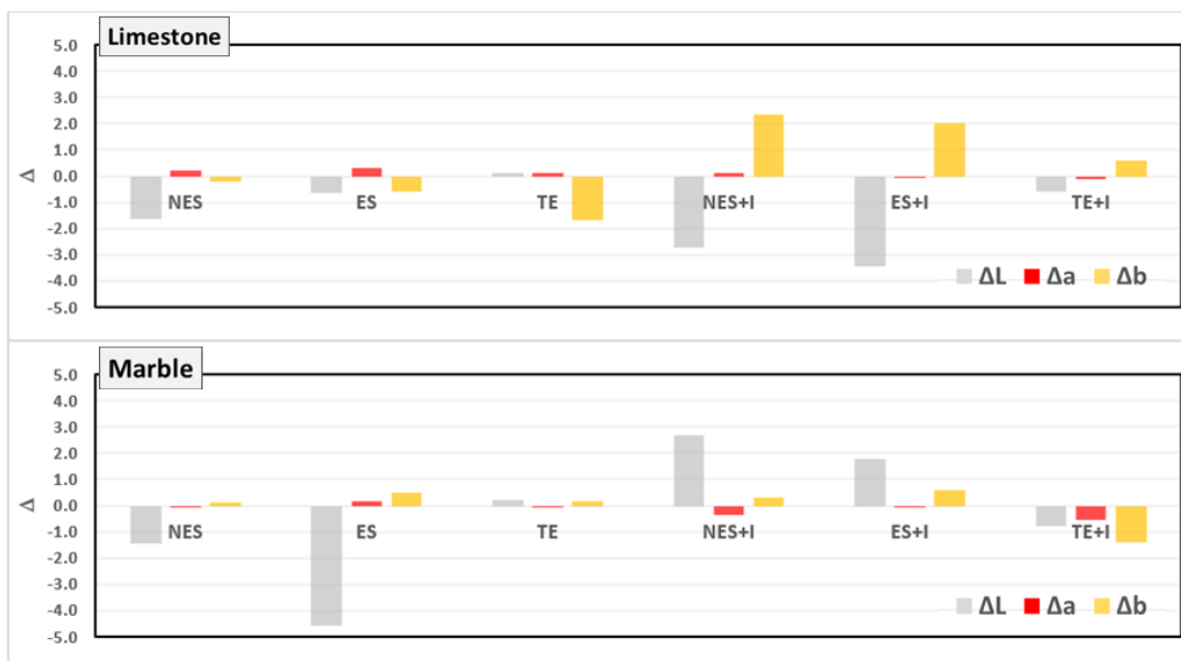
Figure 4. Components \Delta L , \Delta a , \Delta b of \Delta E value for each treatment.
