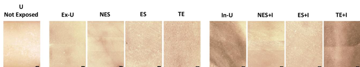
Figure 20. Stereomicroscopy images of untreated and treated marble probes exposed for 24 h, Mag. 26 ×, bar. 1 mm.
