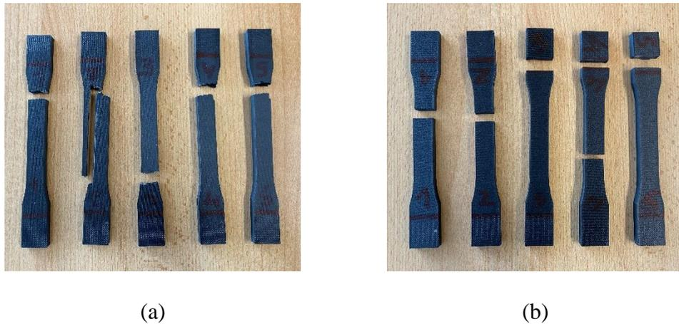
Figure 27: (a) Failure modes under tensile load for chopped FRP- $0^\circ$ ; (b) failure modes under tensile load for chopped FRP- $90^\circ$
