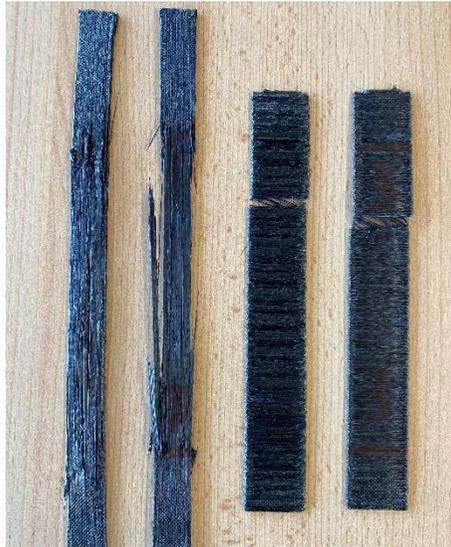
*Figure 34: Tensile failure modes of continuous FRP,  $0^\circ$  (left); tensile failure modes of continuous FRP,  $90^\circ$  (right)*
