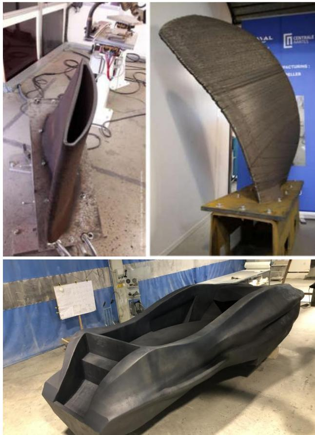
Figure 10: Examples of RAM for marine applications
