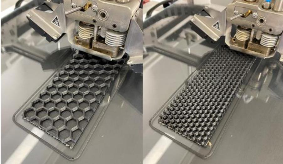
*Figure 41: Additive manufacturing process of AMHSR*
