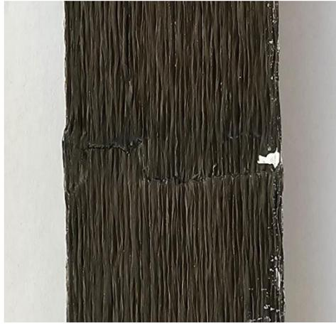
Figure 54: Specimen indentation for  $t_f=2.4$
