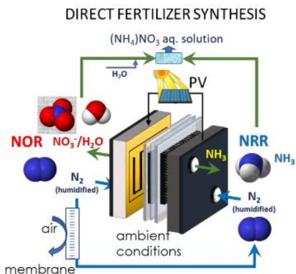
Figure 1.11 Concept of a compact photochemical for a distributed production of fertilizers. From ref [63]
