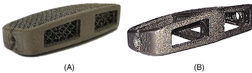
FIGURE 1 Devices object of the study: (A) with porous micro lattice core; (B) without porous micro lattice core
