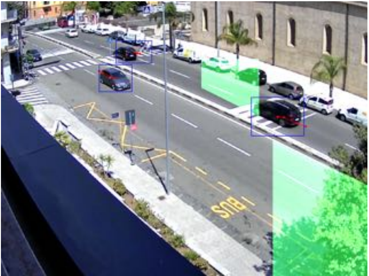
Figure 3.4: Captured frame with moving objects identified. Objects hitting the green area are counted as moving objects.
