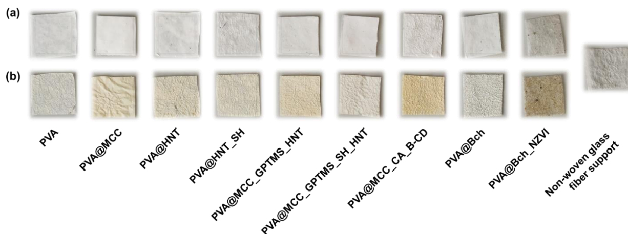
Figure 3.10. The appearance of the produced electrospun nanofiber composite membranes before (a) and after heat treatment b).
