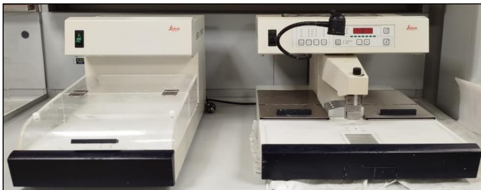
Figure 3.3 Refrigerated counter (left) and inclusion control unit (Leica, Milan, Italy).
