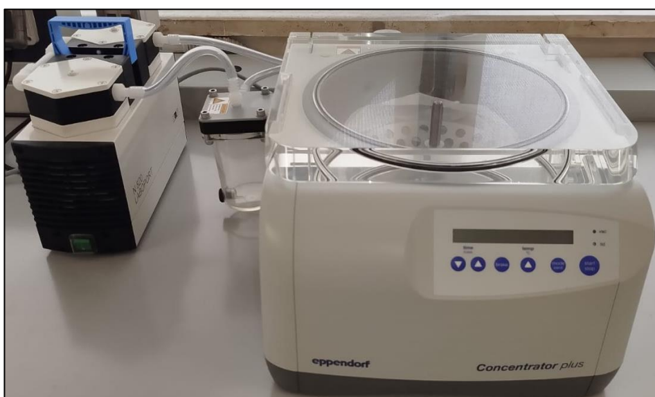
Figure 3.7 Concentrator plus with vacuum pump (Eppendorf, Milan, Italy).
