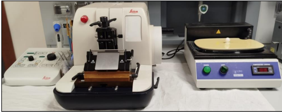
Figure 3.4 Automatic rotating microtome and thermostatic bath (right) (Leica Microsystems, Wetzlar, Germany).
