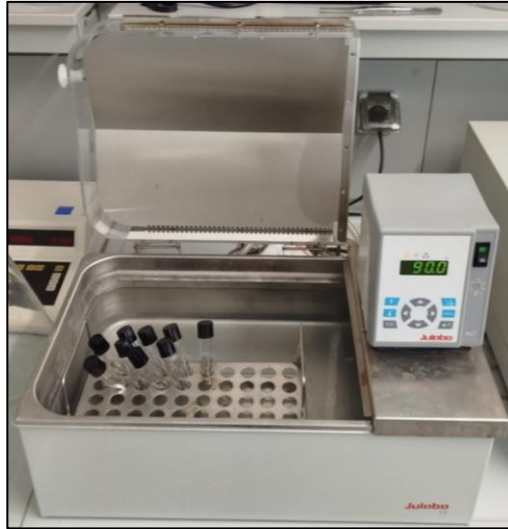
Figure 6.8 Thermal bath (Julabo, Milan, Italy).
