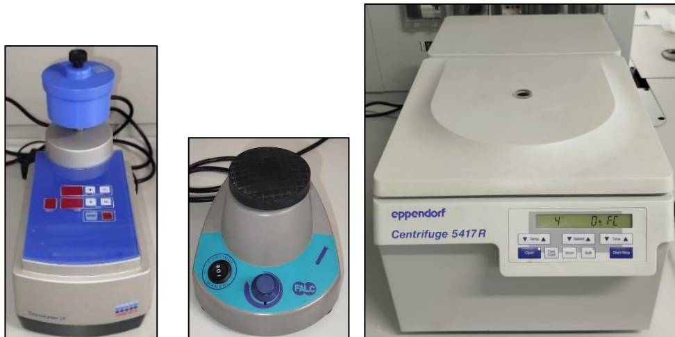
Figure 3.6 In order: TissueLyser LT (Qiagen, Hilden, Germany), vortex mixer (Falc, Perugia, Italy) and centrifuge 5417R (Eppendorf, Milan, Italy).
