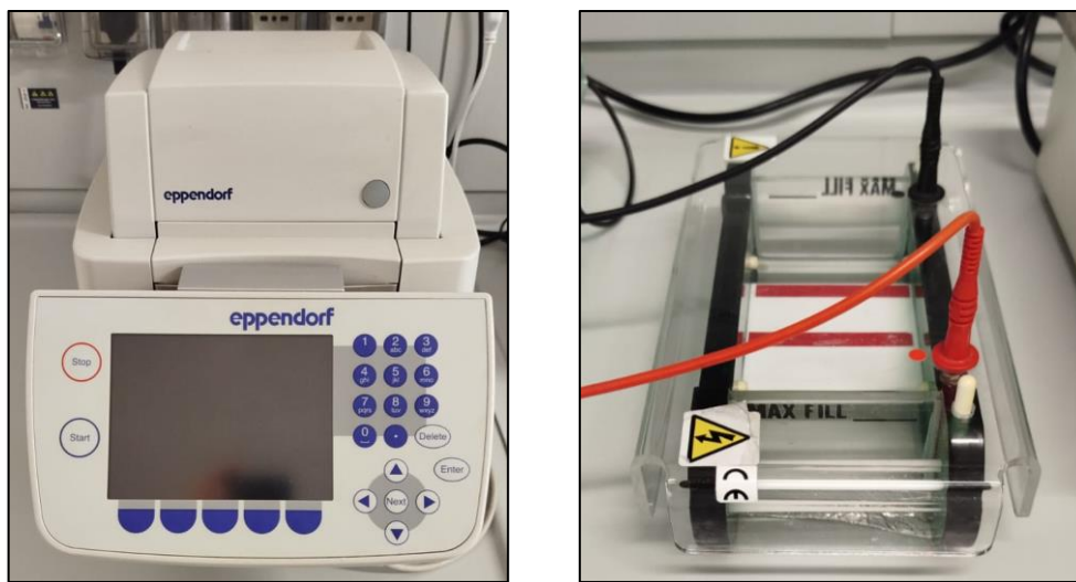
Figure 4.6 Thermocycler (Eppendorf, Milan, Italy) (left) and electrophoresis run tray (right).
