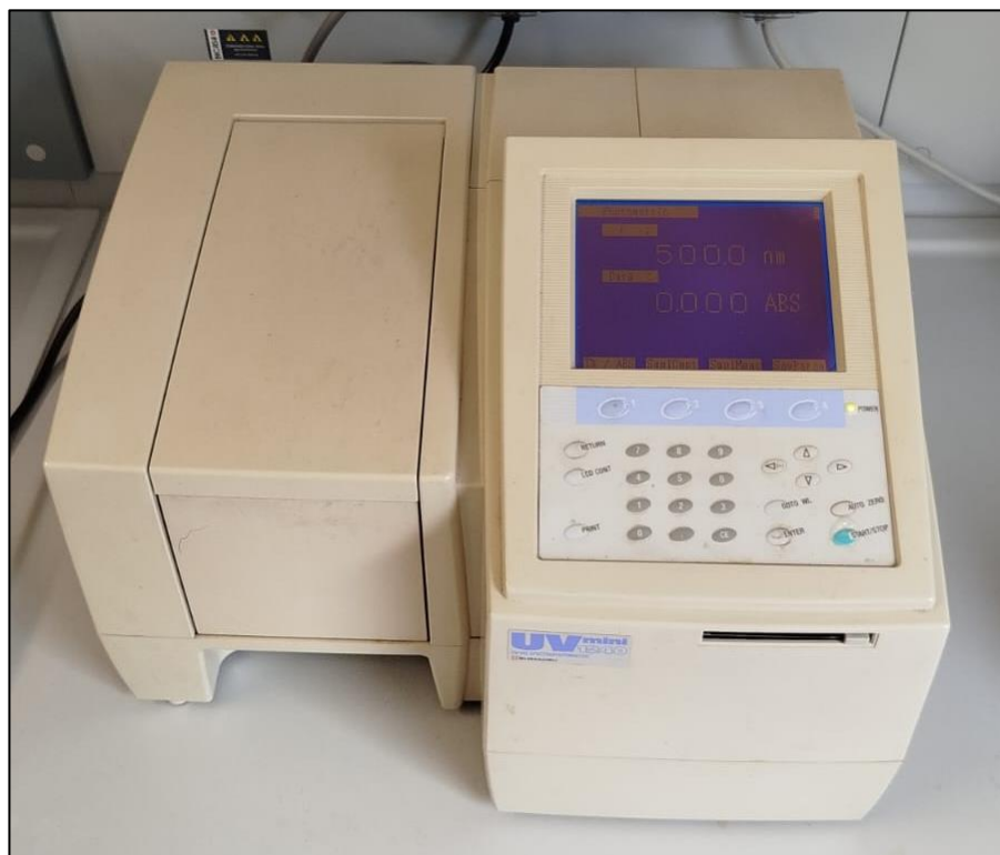
Figure 6.7 UV-mini 1240 spectrophotometer (Shimadzu, Milan, Italy).
