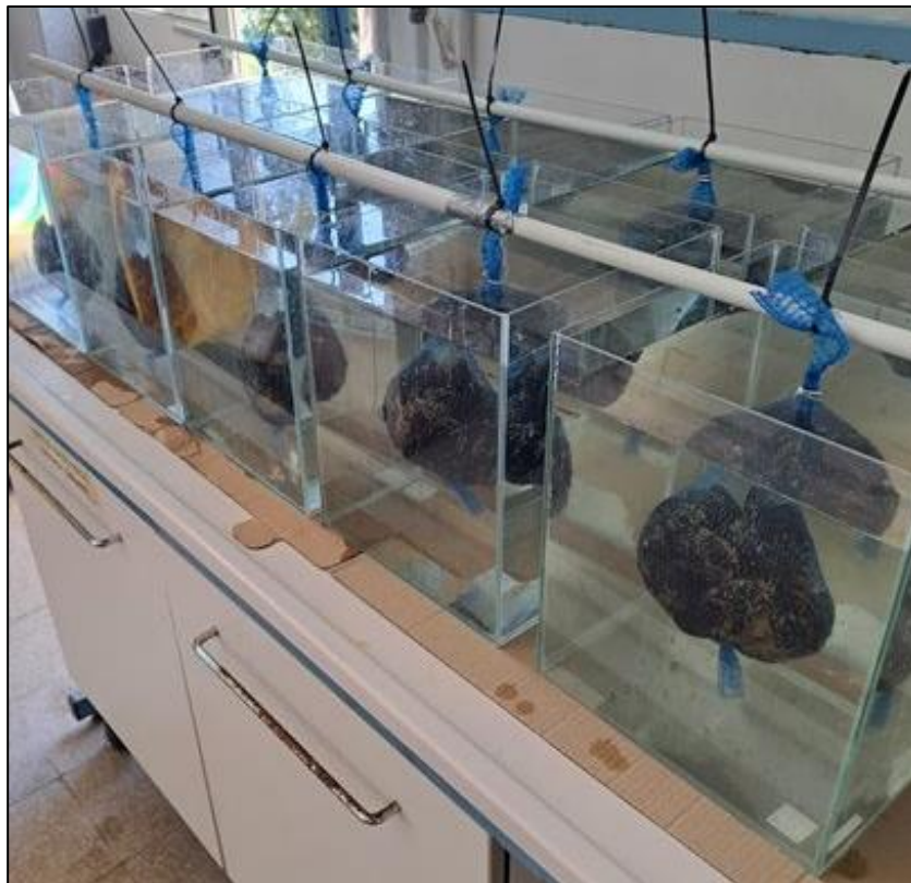
Figure 4.5 Set up of the experimental plan in duplicate in which it is possible to see the glass tanks used for each condition (C0: 0 \mu\text{g/L} , C1: 0.004 \mu\text{g/L} Dex, C2: 0.04 \mu\text{g/L} Dex, C3: 0.4 \mu\text{g/L} Dex and C4: 2 \mu\text{g/L} Dex), with the specimens of M. galloprovincialis allocated.
