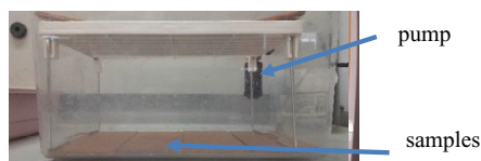
Figure 6. Shipbuilding steel probes coated with different coatings into an aquarium tank with a recirculating pump.
