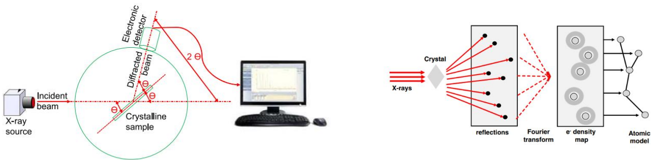
Figure 4.4. (a) Schematic representation of XRD instrument; (b) Basic principle of XRD.
