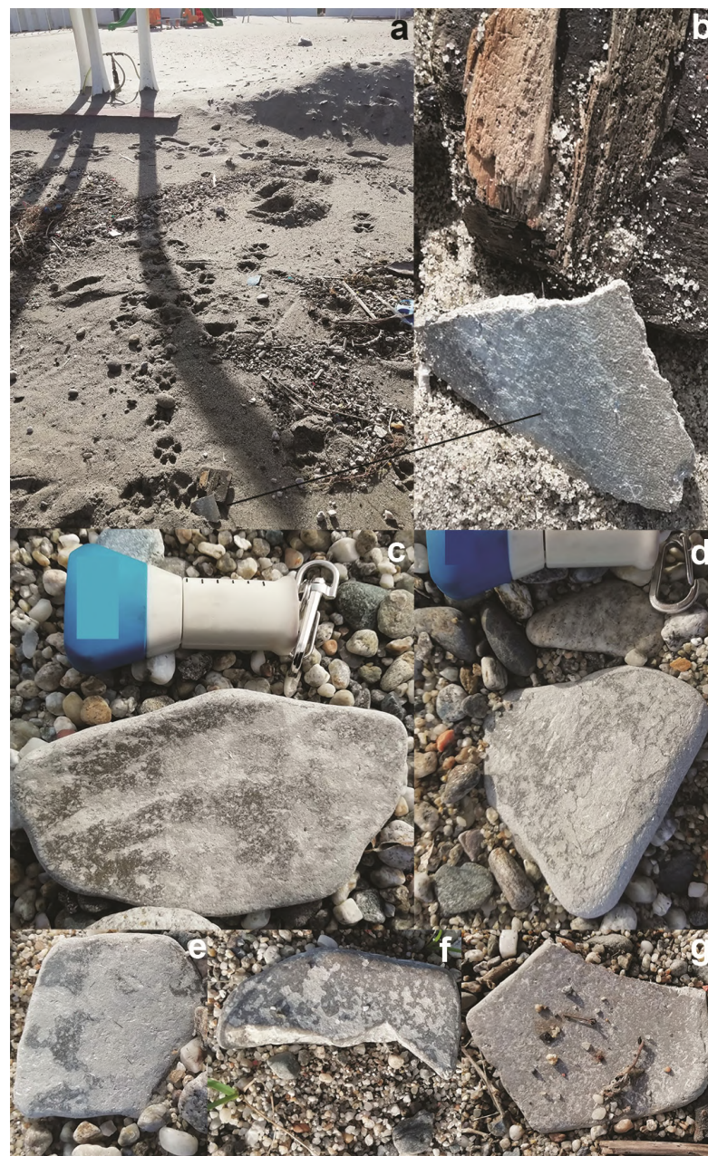
Figure 5. Evidence of ACMs in control sites. (a,b) A decimeter size and angular fragment of ACM in a resort of the Tyrrhenian coast, neighboring the O.N.R. at Mortelle (Lat.: 38^{\circ}16'19.44'' N, Long.: 15^{\circ}37'54.42'' E). (c–g) Well-rounded fragments, partly broken, found on a beach along the Ionian coast, at Sant’Agata (Lat.: 38^{\circ}15'7.95'' N, Long.: 15^{\circ}35'56.18'' E). Source: Authors.
