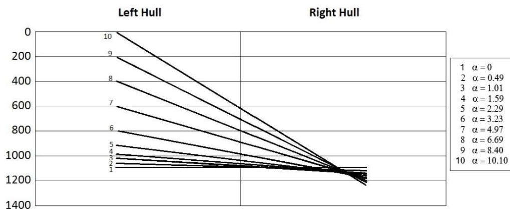
Figure 3. Immersion of the hulls as a function of the heeling angle ( \alpha deg.).
