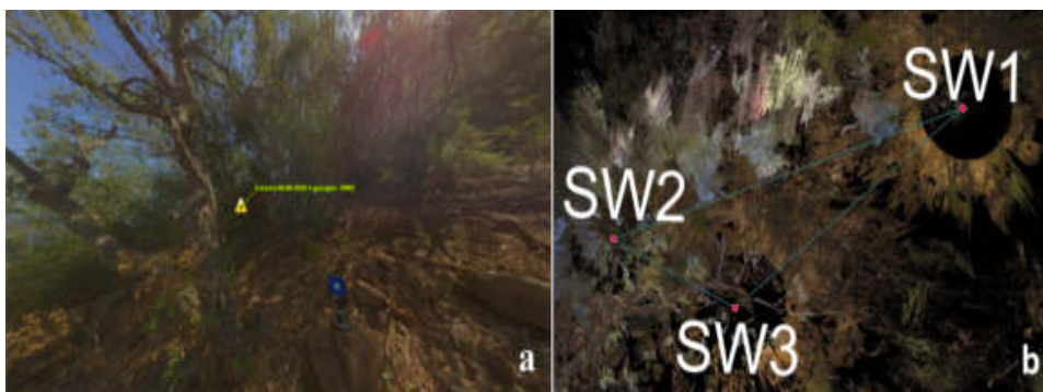
FIGURE 4. Case study 2. a) Photograph of some areas of the scene. b) Orthographic view of the point cloud of case study with stations. 2. Symbol: the red dot indicates the station of measure of the scanner.
