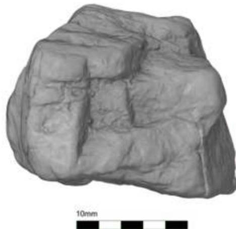
FIGURE 10. Reconstruction of the specimen of case study 5. 3D virtual model related to a block of quartzarenite acquired by means of the blue structured light technology in laboratory. The model allows to observe details present on the surface such as the two systems of joints cross-cutting the rock.
