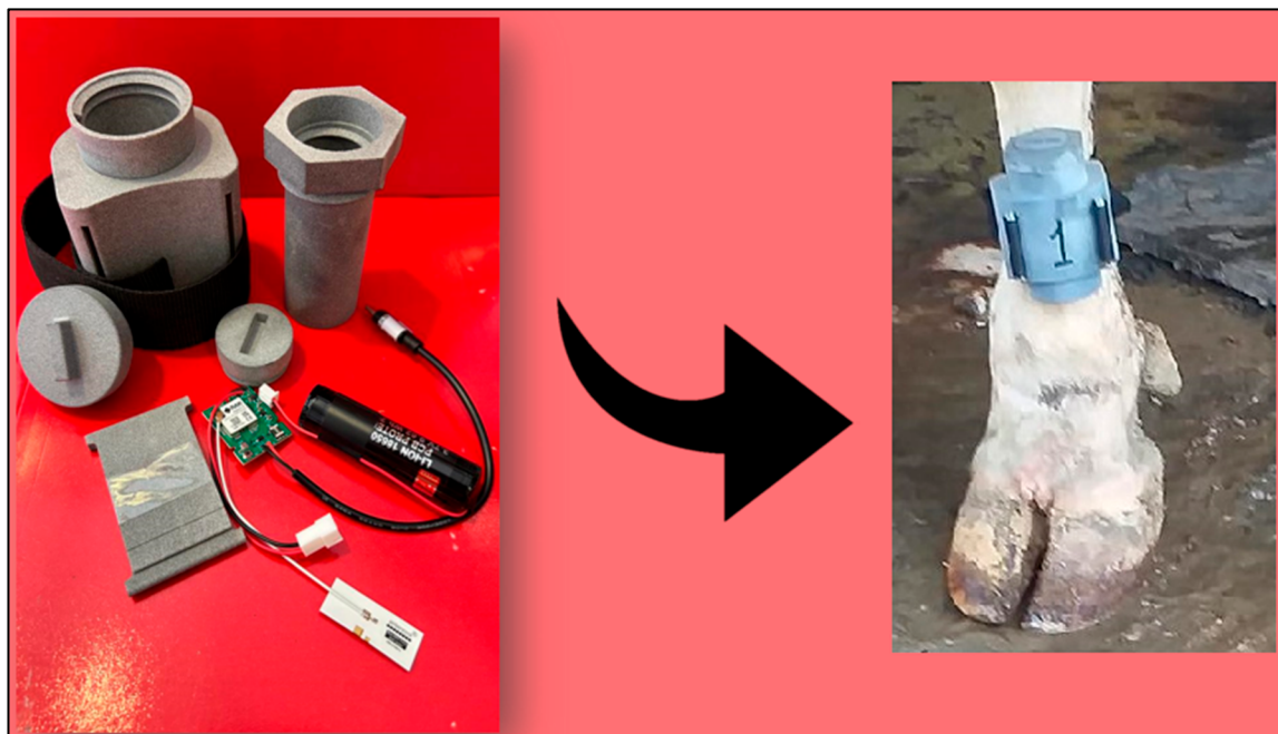
Figure 2. Components and SASP mounting on the cow foreleg.
