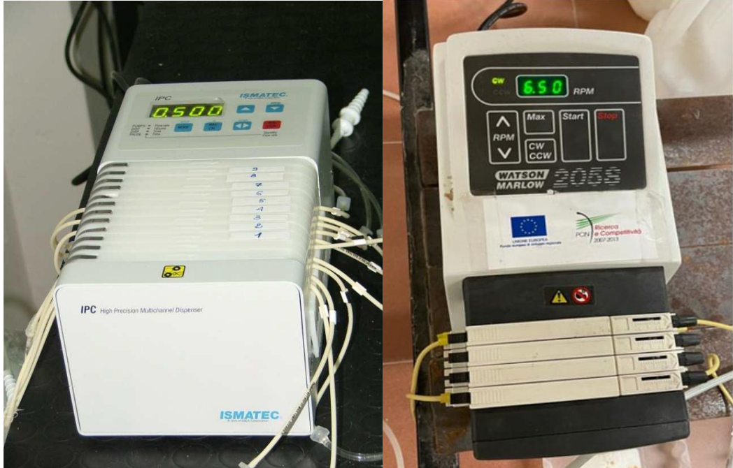
Figure 2.11 Peristaltic pumps: a) Ismatec IPC 12; b) Watson Marlow 205S.
