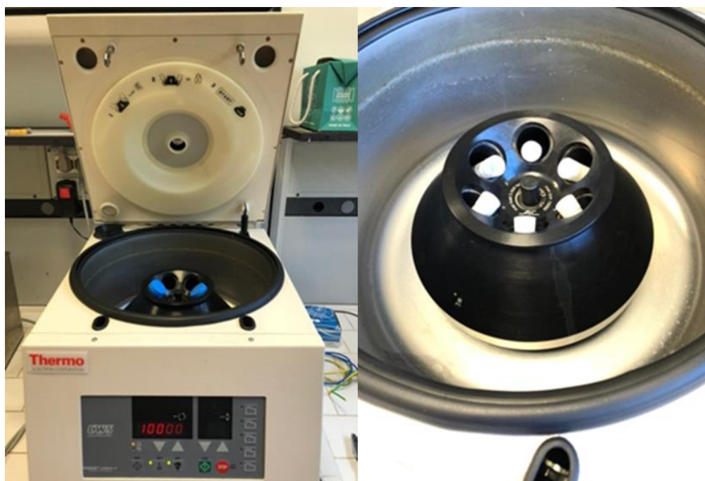
Figure 2.14 ALC-PK 121 centrifuge, internal with detail of the specimens.
