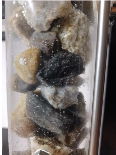
Figure 4.2 Presence of gas bubbles at the beginning of the test.
