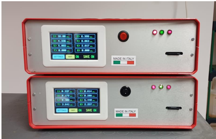
Figure 2.10 Automated system for saving the signals from pressure transducers.
