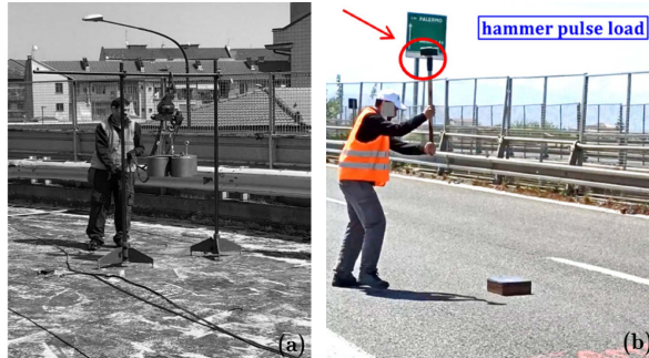
Figure 1.7: Type of excitation in a free vibration test: (a) free falling mass [42]; (b) hammer impulse excitation [43].
