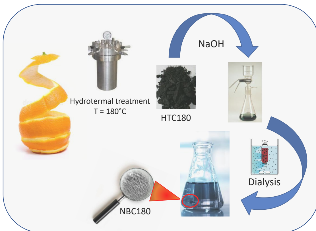
Figure 3.3.1. Illustration outlining the process for synthesizing NBC 180
