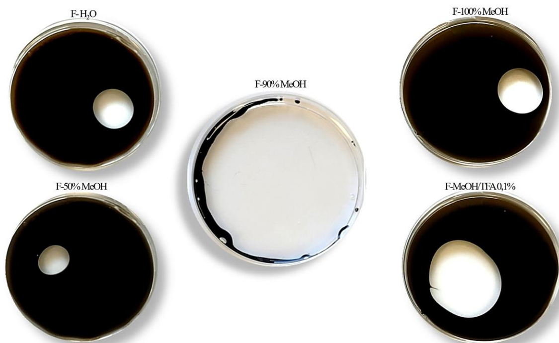
Figure S1. Surfactant activity evaluation of SPE fractions from Bacillus sp. BCP32 by oil spreading test. DMSO (4 \mu L) was used as negative control. The clear zone on the oil surface indicates the presence of biosurfactants. F-90% MeOH showed the best surfactant effect.
