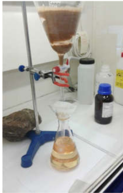
Figure 10. Separation of the heavy minerals from the light ones using diiodomethane ( \text{CH}_2\text{I}_2 ), filters, and laboratory glassware under a chemical fume hood. Source: own development.
