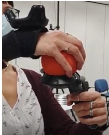
Figure 3.12. Hand-ball distance calibration. The figure shows the calibration procedure required to estimate the participant-dependent distance between the ball and thrower's hand.
