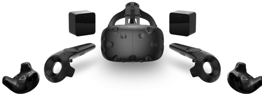
Figure 3.2. Htc Vive system. The system consists of the headset to display VR, 2 base stations, 2 controllers and 2 trackers for motion capture.
