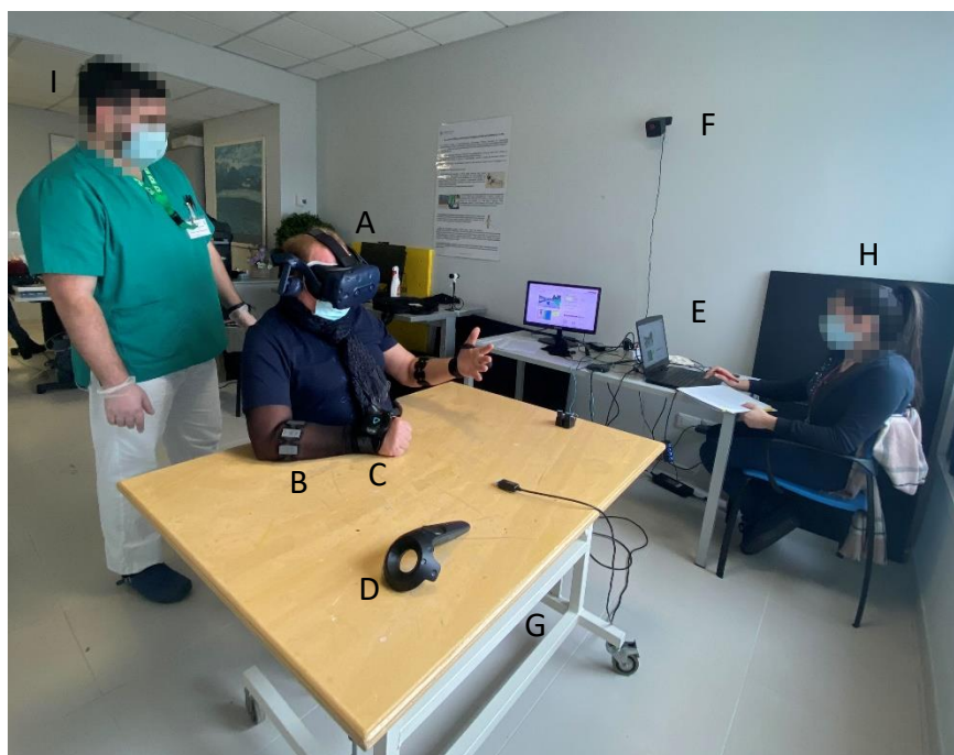
Figure 4.1. VVita Setup. (A) Virtual reality headset HTC Vive. (B) EMG bracelet Thalmic labs Myo. (C) Motion capture HTC Vive tracker sensor. (D) Motion capture HTC Vive controller sensor. (E) Laptop connected to the system. (F) One of the two HTC Vive base stations. (G) Adjustable table. (H) Therapist. (I) Physiotherapist.
