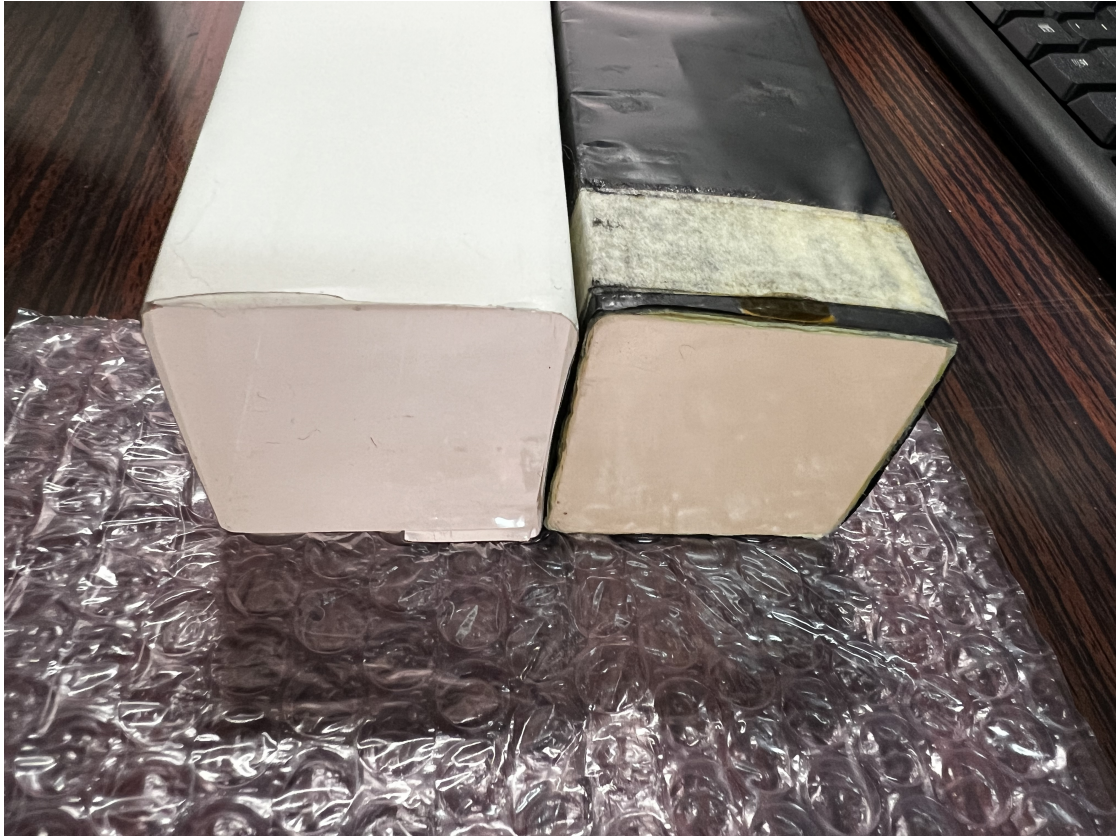
Figure 54: Visual effect of polishing. On the left is polished crystal, and on the right, the original BaBar one
