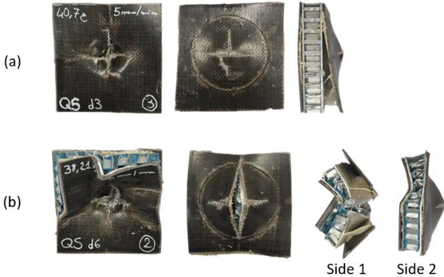
Figure 60: Visual inspection of failed BFRP/AHS panels after QS perforation: (a) BFRP/AHS d3 specimen, (b) BFRP/AHS d6 specimen.
