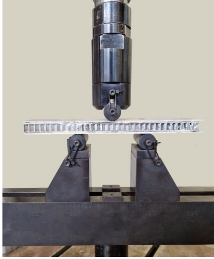
Figure 39: Three-point bending test setup for FFRP/AHS panels [170].
