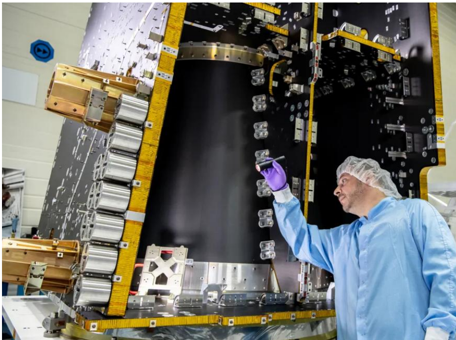
Figure 17: Example of a satellite sandwich structure (Image from www.beyondgravity.com ).
