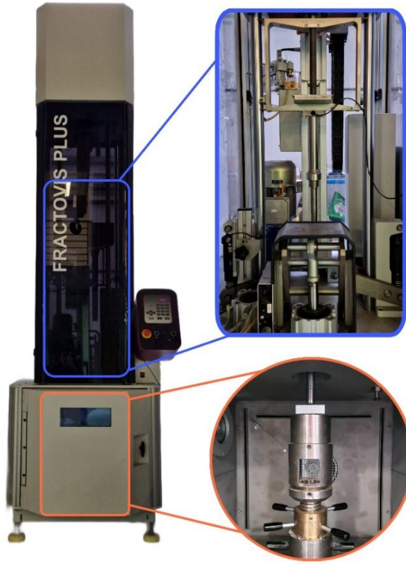
Figure 23: CEAST FRACTOVIS drop test machine [168].
