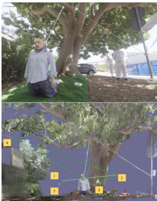
FIGURE 4. Case study 1. Different view of the 3D virtual model of the simulated crime scene where the victim was simulated by a hyper-realistic dummy. The red spheres indicated the position of the stations.
