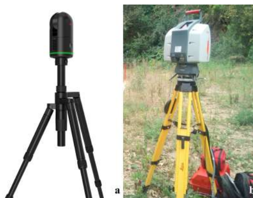
FIGURE 2. Laser scanners: Leica BLK 360 model (a) and Leica Nova MS50 MultiStation (b) of the Department of Engineering of the University of Messina.
