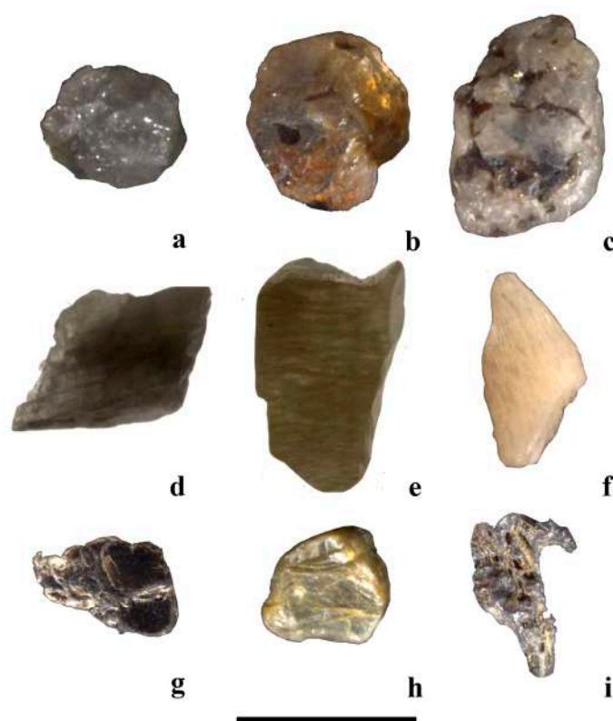
Figure 4. Main types of mineral grains forming the sands (Sample TB01, 1–2 mm sandy fraction), observed under stereomicroscope. (a) Quartz. (b,c) Polymineralic grain of quartz + feldspar + biotite gneiss (b) and augen gneiss (c). (d–f) Monomineralic grain of feldspar showing typical cleavage, and pinkish color in (f). (g) Monomineralic grain of biotite showing typical black color and cleavage. (h) Monomineralic grain of muscovite showing typical white color and cleavage. (i) Volcanic grain with vesicular texture. Reflected light in (a–c,g–i). Transmitted light in (d–f). Scale bar: 1000 \mu m.
