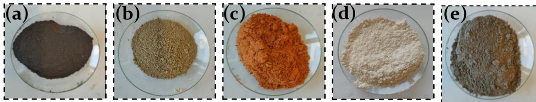
Figure 2.2. Starting materials: (a) DS, (b) clay, (c) BW, (d) K and (e) Slag.
