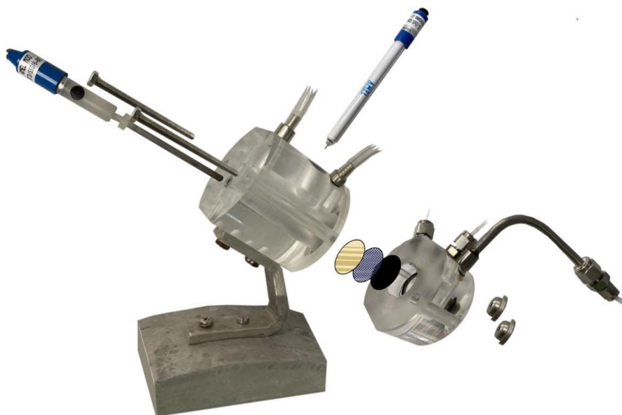
Figure 3.3 – Exploded depiction of the cell
