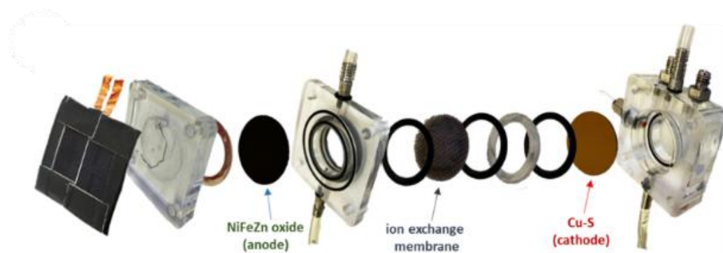
Figure 6.2 - Exploded view of the electrochemical (EC) – photovoltaic (PV) device and related electrodes, including O-rings and gaskets
