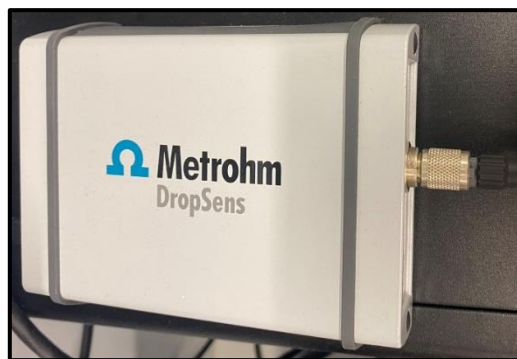
Figure.II. 16. DropSens \mu Stat 400 Potentiostat system at LabSensor for the electrochemical test
