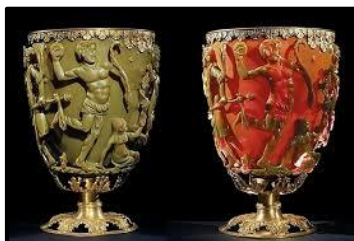
Figure.I. 18. Cup of Lycurgus; in the right is enlightened by transmission and in the left by reflection
