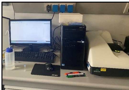
Figure.II. 13.The used DLS spectroscopy at LabSensor
