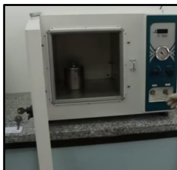
Figure.I. 16. Hydrothermal autoclave reactor into furnace
