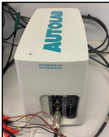
Figure.II. 18. Autolab PGSTAT204 system used for EIS study at LabSensor
