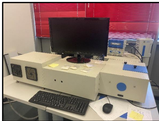
Figure.II. 11.The used PL spectroscopy at LabSensor
