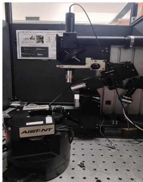
Figure.II.7. Illustration of an Atomic Force Microscope (AFM) contact mode at IPCF-CNR.
