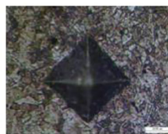
FIGURE 11 Micro-hardness measurement for AM and traditional AISI 316L [Colour figure can be viewed at wileyonlinelibrary.com ]
