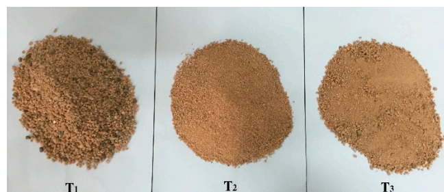
Figure 3. The soil sample (the tailings of ionic type rare earth leached in situ).
