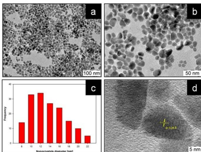
Figure 1. (a, b, d) TEM images of the CuIn $_{0.8}$ Ga $_{0.1}$ Se $_{2.3}$  nanocrystals at different magnifications (c) statistic distribution of the mean nanocrystal diameter.
