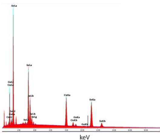
Figure 3. EDX spectrum of  $\text{CuIn}_{0.8}\text{Ga}_{0.1}\text{Se}_{2.3}$  nanocrystals.
