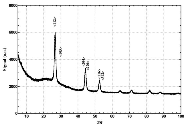
Figure 2. XRD pattern of CIGS nanocrystals.
