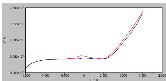
Figure 6. Linear sweep voltammetry (LSV) of a CIGS thin film deposited on ITO coated glass recorded with simulated solar light (red line) and under dark condition (black line).
