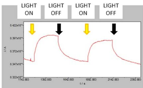
Figure 5. Transient photocurrent response of a CIGS thin film deposited on ITO glass substrate, recorded during two cycles of on-off made by irradiating the sample with simulated solar light.
