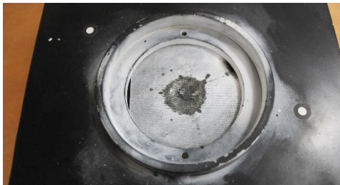
Figure 2- The specimen inside the clamping system. It is possible to note the markers for the 3D scanner
