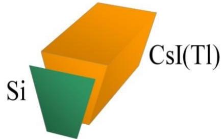
Figure 2.2: The basic detection module of CHIMERA apparatus.
