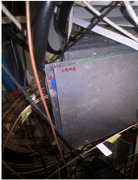
Figure 4.11: ASAD cards with aluminum shields. These provisional shields will be replaced by the ones shown in Figure 3.12.
