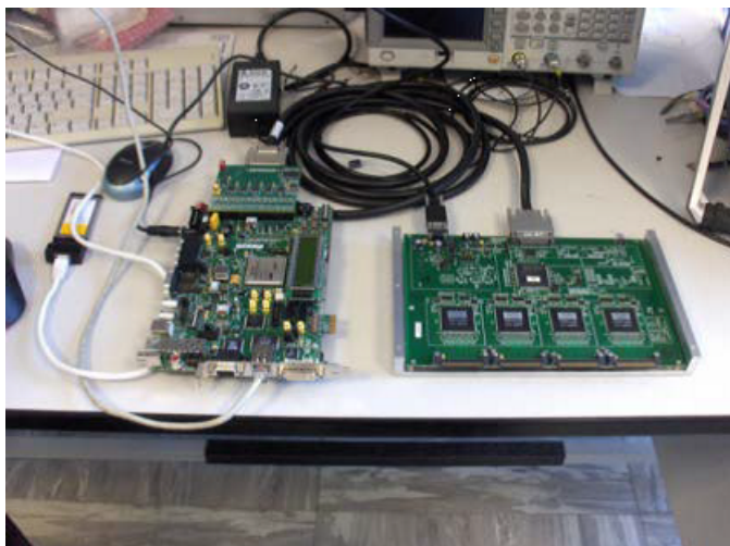
Figure 3.5: The test system with one ASAD card and the Reduced CoBo.
