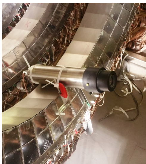
Figure 4.21: The experimental set-up for the test of the EJ 299 – 33 plastic scintillator. The scintillator coupled to photomultiplier covered by black plastic can be observed between Ring9 and the sphere of CHIMERA.
