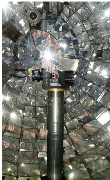
Figure 2.11: Reflecting system of the laser beam positioned in CHIMERA vacuum chamber during various tests at LNS.
