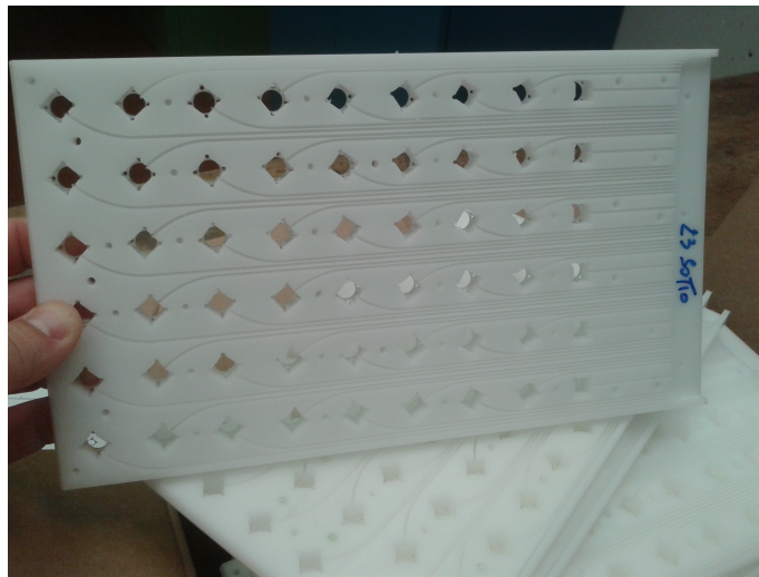
Figure 5.12: Picture of the g-2 front panel. Each hole in the delrin plate houses a 8 \times 8 \text{ mm}^2 45^\circ prism which deflects the light coming from the fiber placed inside the groove.
