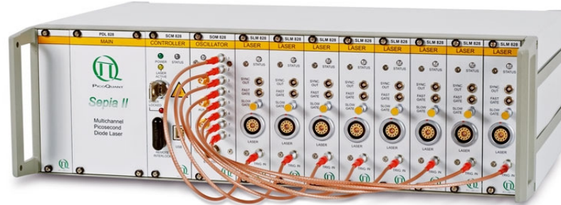
Figure 5.8: Laser crate “Sepia”. Each laser head LDH-P-C-405M will be coupled to its driver (the crate contains up to 8 drivers).
