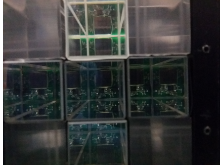
Figure 6.2: A front view of the calorimeter. Different crystal wrappings can be observed (top crystal in white wrapping). It is possible to recognize the real crystal from the fake Plexiglas ones, looking at the SiPM image reflected on the rear side.
