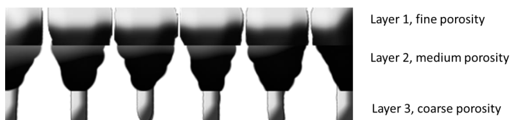
Figure 3 - Asymmetric Membrane Concept (layer 3 is usually intended as a mechanical support for the medium and fine porosity layers)
