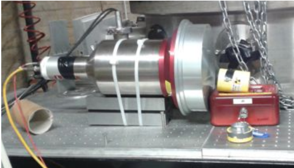
fig. V- 11 Photography is shown in the scintillator EJ301 coupled with phototube; the radioactive source of Am-Be placed on the red box is visible
