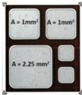
fig. V- 34 SiC detectors with different area A = 1 \text{ mm}^2 and 2.25 \text{ mm}^2
