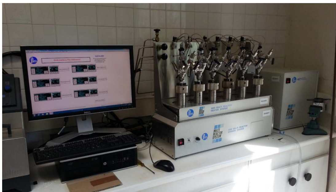
Figure 2.2 Parr 5000 Multiple Reactor System and Control Unit
