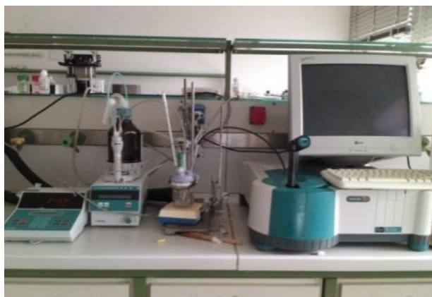
Figure 4.7. Varian Cary 50 UV–Vis spectrophotometer and the apparatus used for the experiments.
