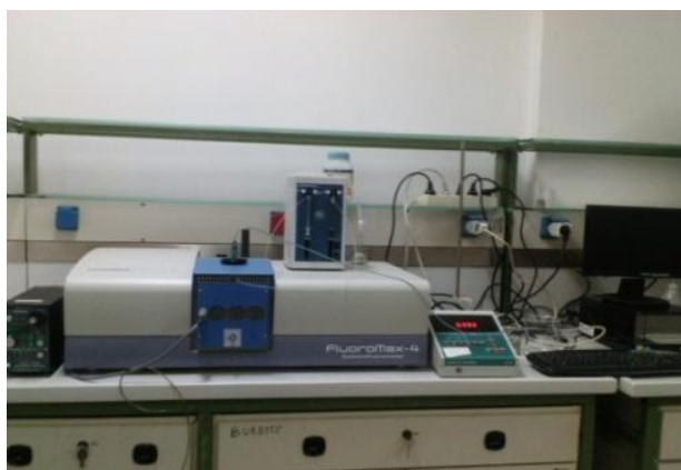
Figure 4.10. FluoroMax-4 spectrofluorimeter and apparatus used for the measurements.
