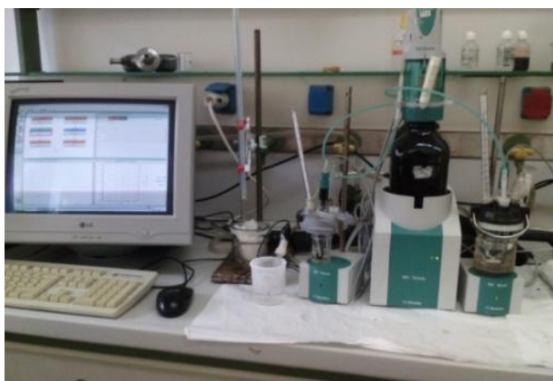
Figure 4.3. Metrohm model 809 Titrando and the apparatus for potentiometric measurements.
