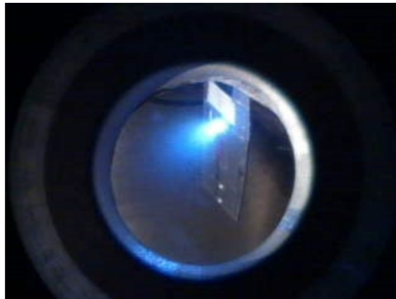
FIGURE 4.2: CCD image of a Cu plasma generated by a Nd:YAG laser.
