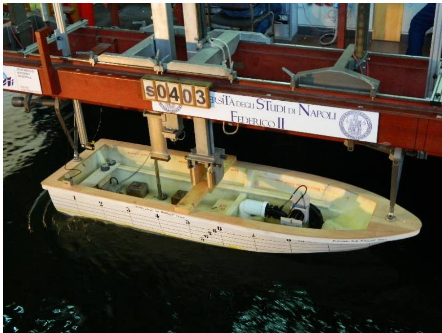
Figure 37 - The hull model in the towing tank
