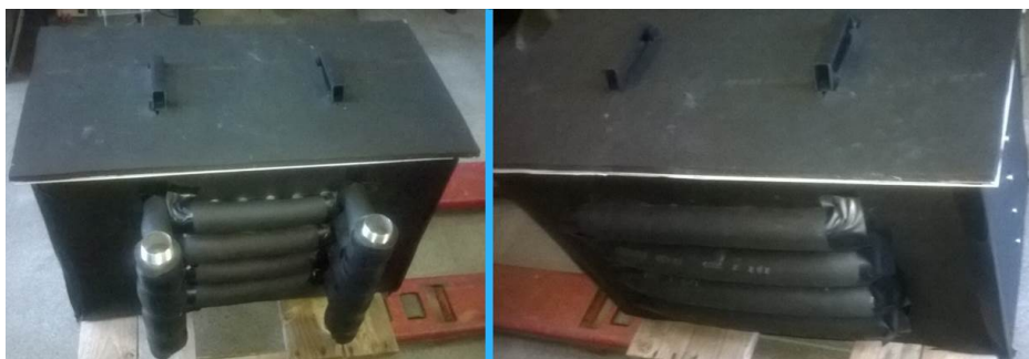
Fig. 3.16 The prototype of TES after the application of the first layer of insulation.
