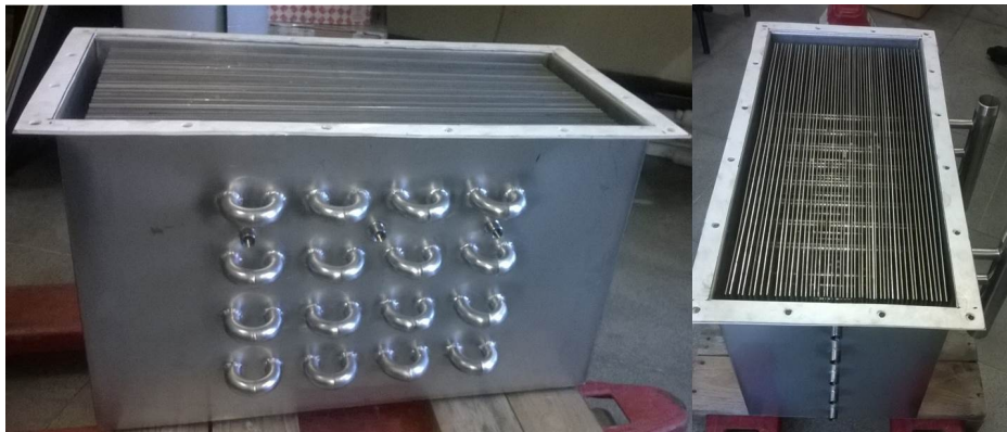
Fig. 3.14 The prototype of fin-and-tube HEX with PCM realised.
