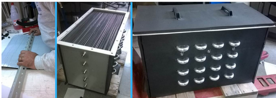
Fig. 3.15 The prototype TES after the application of the first layer of insulation.
