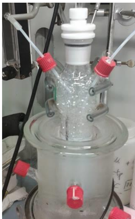
Figure 183. Foam formation in the sonochemical reactor due to surfactant excess
