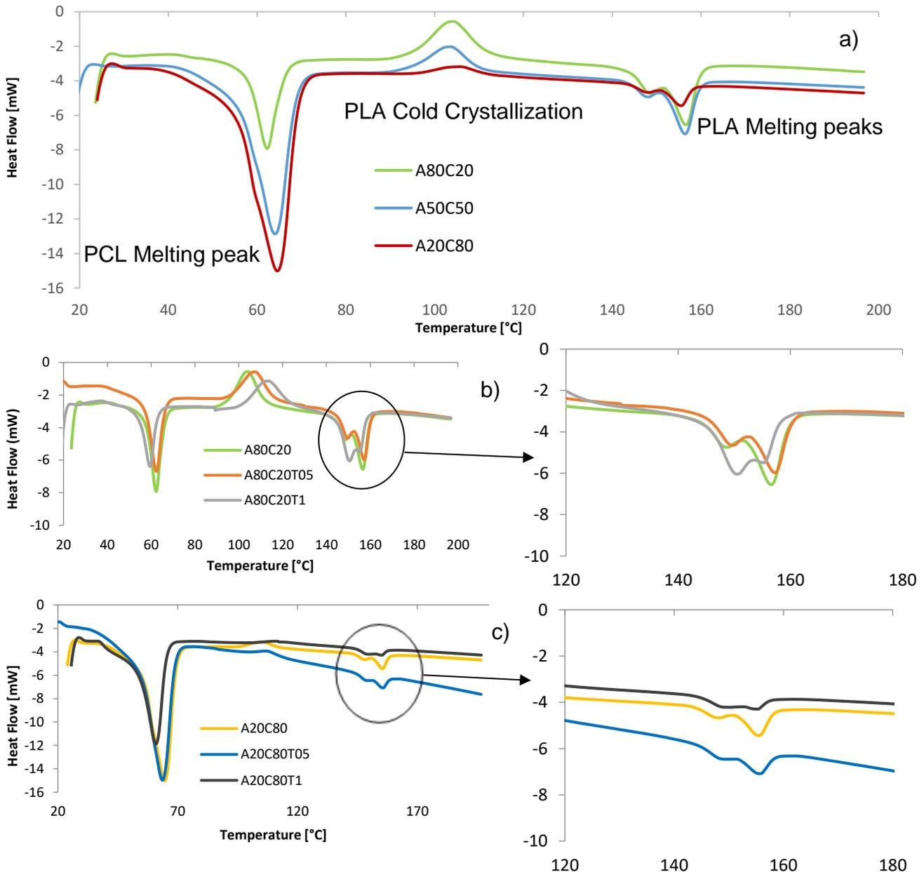
Fig. 5.9 DSC Thermograms of physical (a) and reactive(b,c) blends, Polyester weight ratio effect
