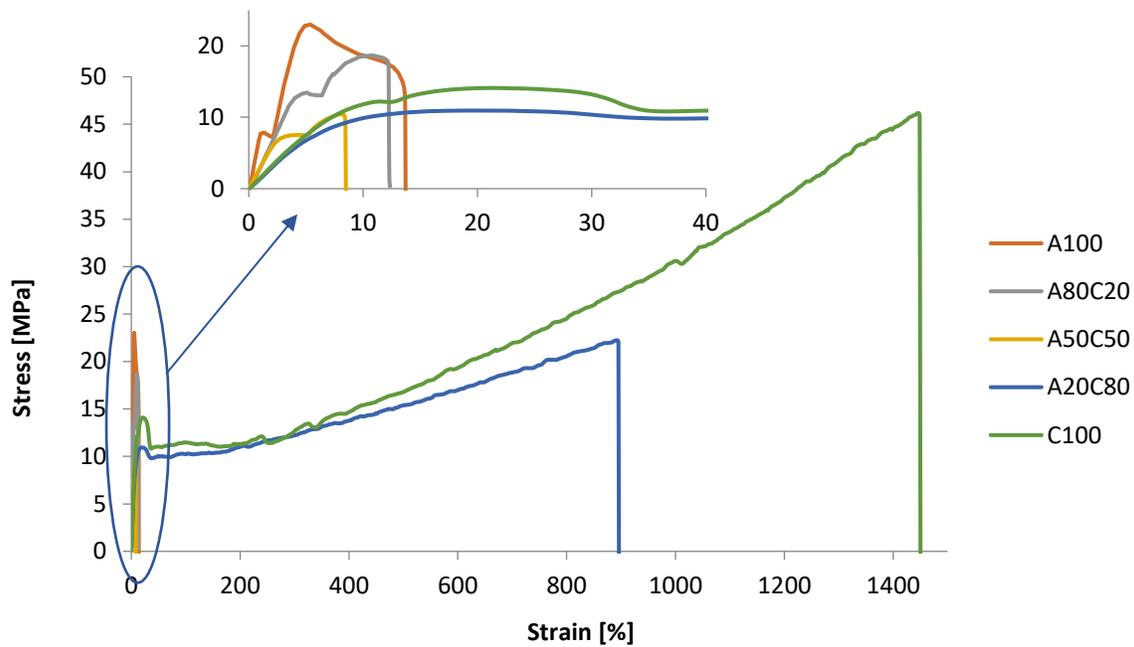
Fig. 5.5-b Physical Blends Stress-Strain Curves
