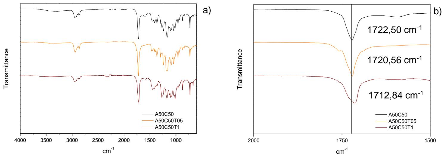
Fig. 5.17 a) FT-IR Spectra of A50C50 physical and reactive blends (0,5 and 1 phr LTI), b) C=O stretching peak zoom
