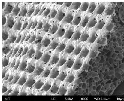
Fig. 1.10 SEM image of a porous polyester scaffold obtained with phase inversion process of polymers with micro patterning. Credit : The Koch Institute Public Galleries (<https://ki-galleries.mit.edu/2016/hyder-2>)
