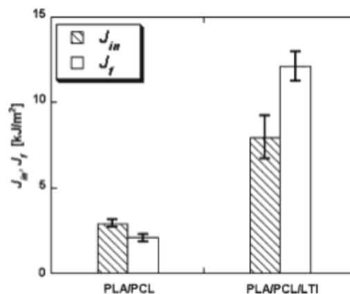
Fig. 3.6, Initial crack ( $J_{in}$ ) and Average fracture energy ( $J_f$ ) for PLA/PCL and PLA/PCL/LTI blends [17]
