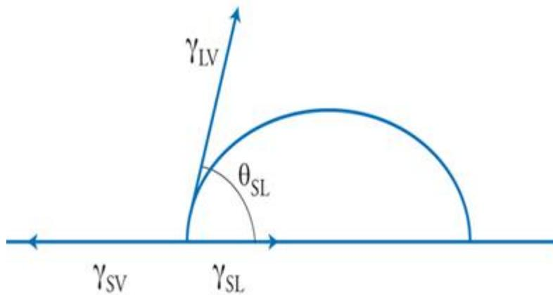
Fig. 4.10 Schematics of the wet-ability measurement test
