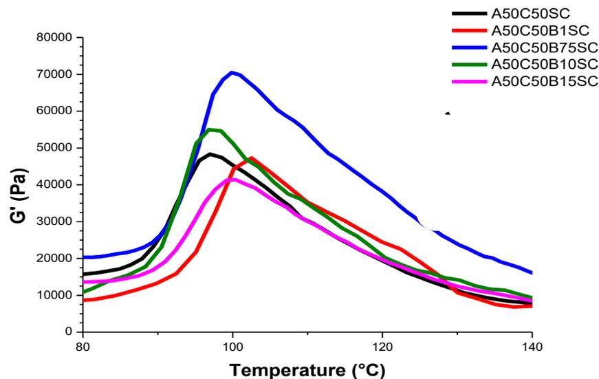
Fig. 5.21 Rheology Temperature ramp test trend of solvent cast blends, PLA Cold Crystallization temperature range
