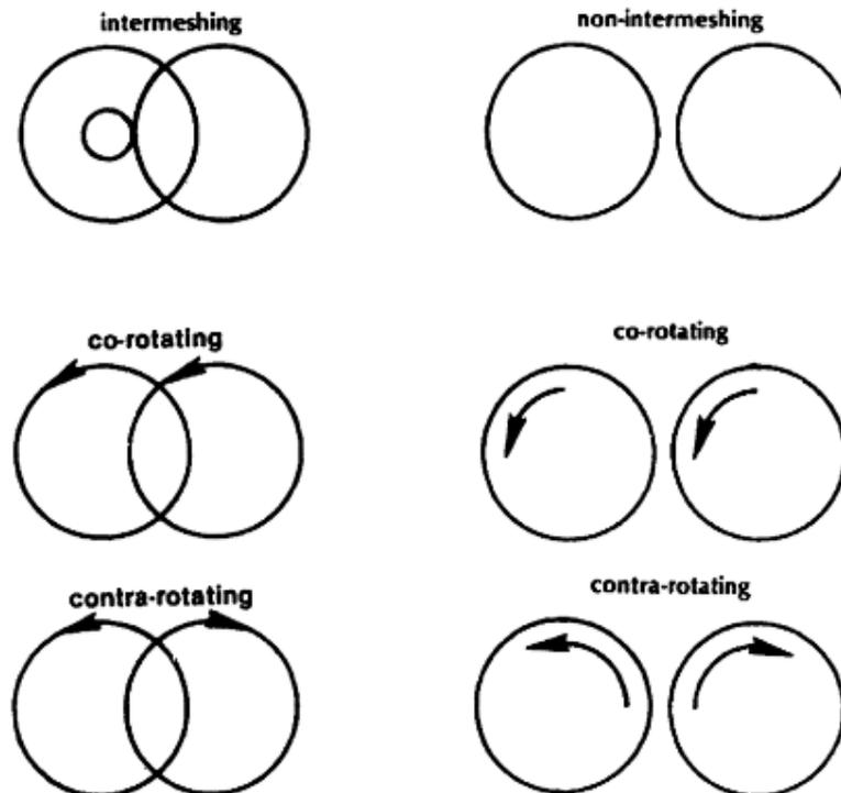
Fig. 2.4 Schematic representation of Twin Screw Extruders Types [7]
