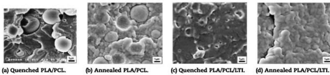
Fig. 3.8 SEM images of quenched and annealed PLA/PCL and PLA/PCL/LTI blends [20]
