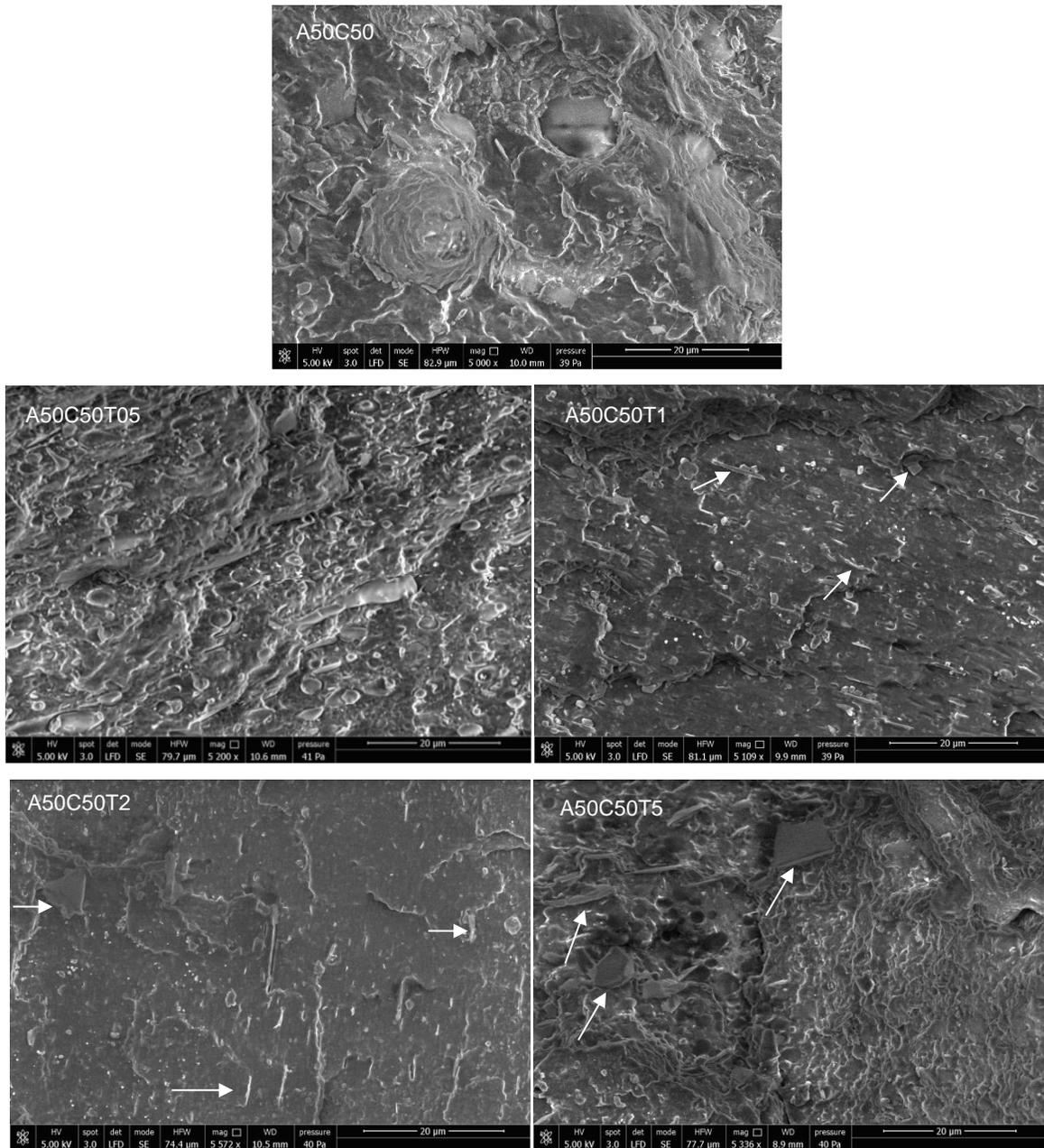
Fig. 5.14 SEM images of physical and reactive blends before rheology tests.
