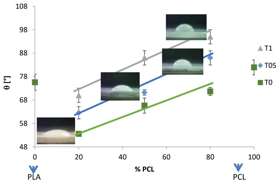
Fig. 5.16, PBS surface angle values of Physical and reactive blends vs PCL weight ratio
