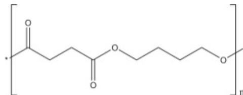
Fig. 1.7 Poly(butylene succinate) chemical structure
