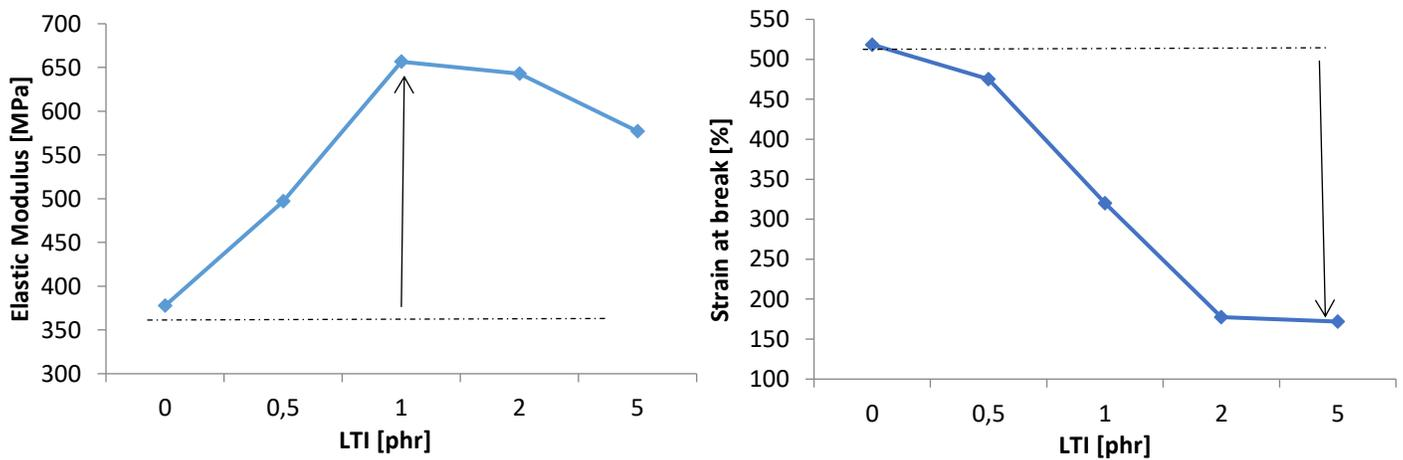
Fig. 5.20 Elastic Modulus and Strain at break vs LTI amount in extruded blends
