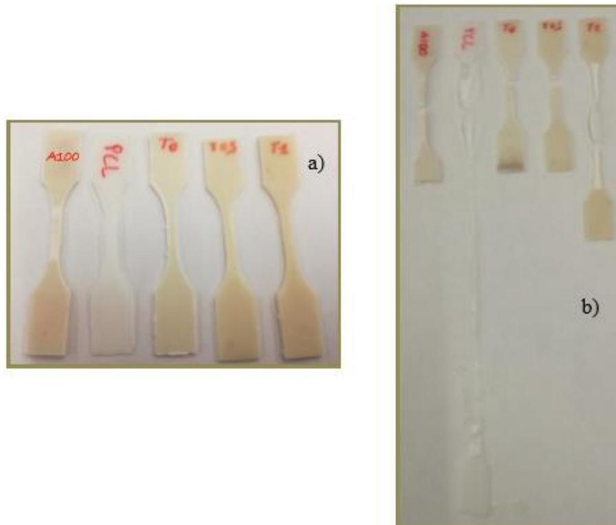
Fig. 5.4 Images of Dog-bone Type V ASTM D638-10 specimens before a) and after b) Tensile tests
