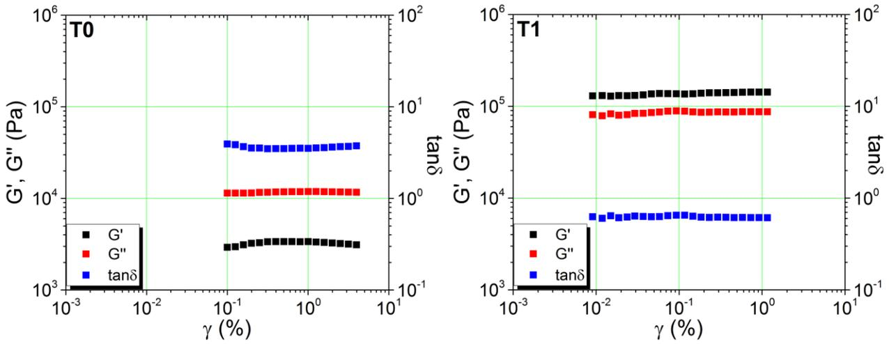
Fig. 5.11, Shear Amplitude variation test of A50C50 and A50C50T1 blends
