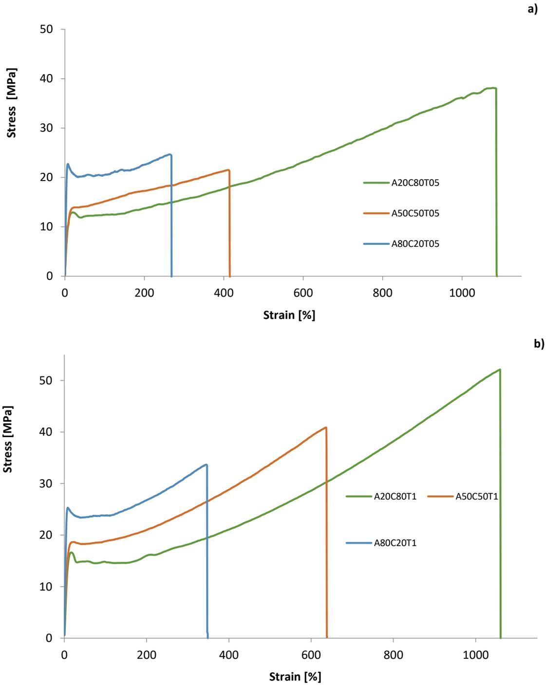
Fig. 5.7 Stress-Strain Curves of physical and reactive blends by composition; a) 0,5 phr LTI b) 1 phr LTI.
