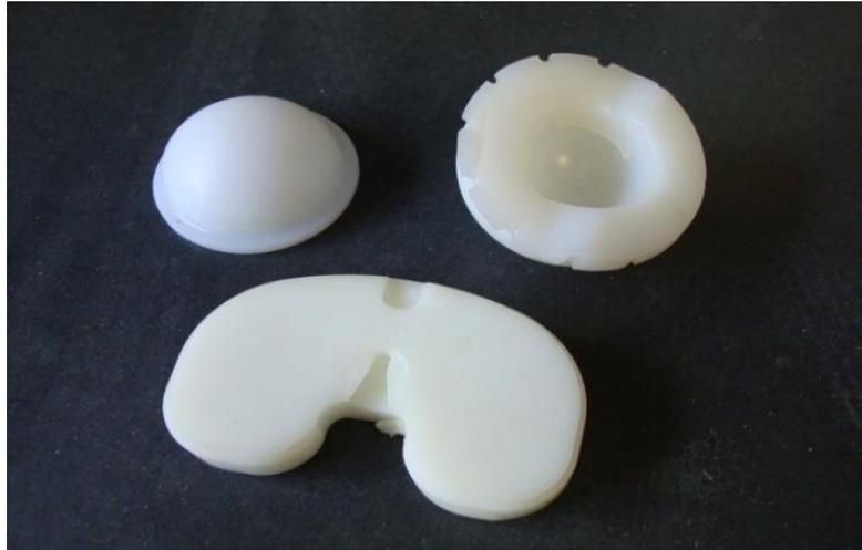
Fig. 1.3 Examples of UHMWPE Joint Replacement parts [8].
