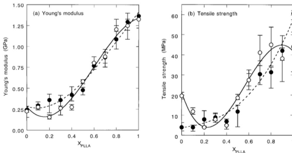
Fig. 3.5, Young's Modulus and Tensile Strength of PLLA/ PCL blends without (black dots) and with (white dots) 10% of PLLA-CL [12]
