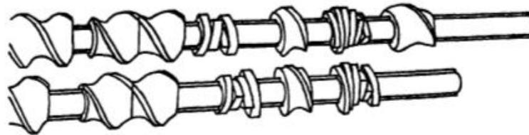
Fig.2.5, Example of design of screws kneading building blocks in compounding
