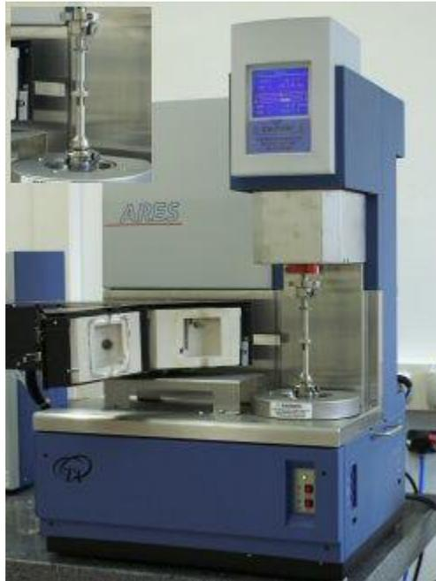
Fig. 4.8 TA Instruments ARES LS2 Rheometer
