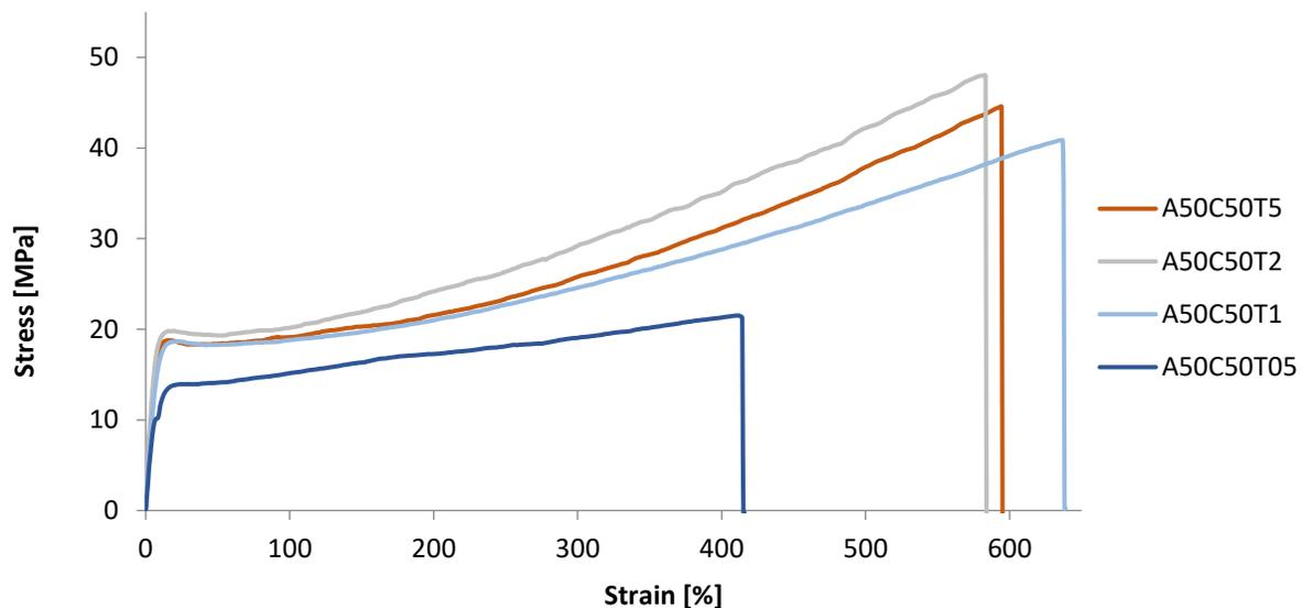
Fig. 5.6 Stress-Strain curves of A50C50 reactive blends
