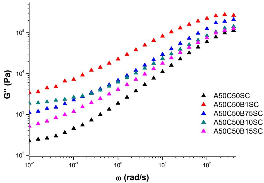
Fig. 5.22 Frequency variation tests trends of Shear Moduli for A50C50 Solution cast blends (top G', bottom G'').
