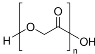
Fig. 1.6 Poly(glycolide) chemical structure
