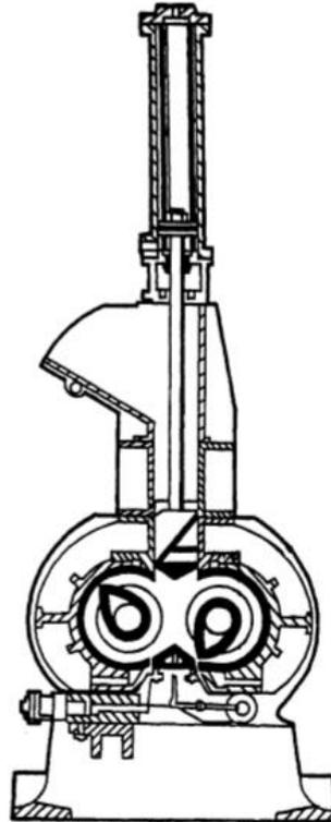
Fig. 2.2, cross sectional view of a batch mixer, [7]
