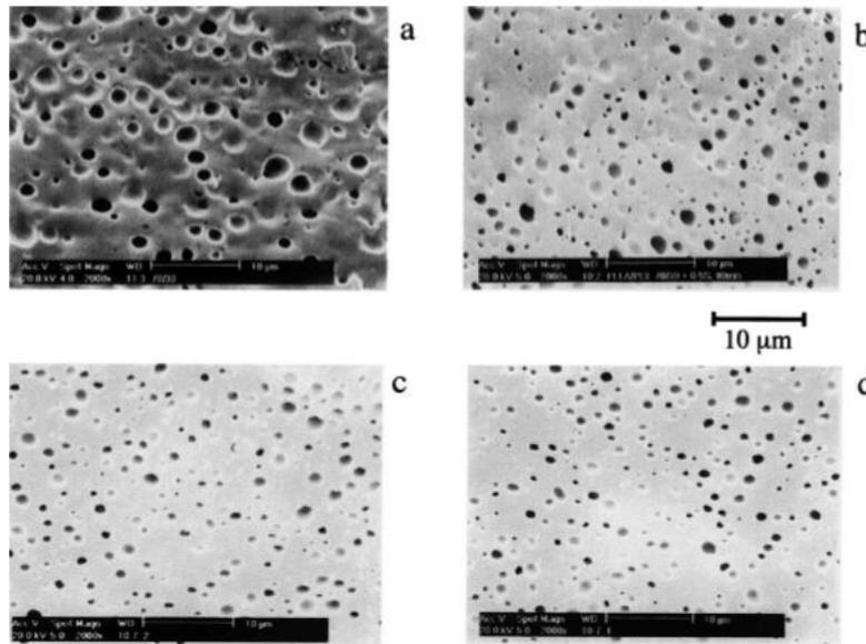
Fig. 3.4, Optical microscopy images of PLA/PCL blends (Wt ratio 70/30) with 0 a), 0.5 b), 2 c), 5 d) phr of PLLA-PCL-PLLA triblock [7]
