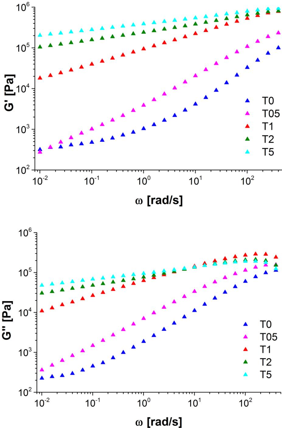
Fig. 5.13 Frequency variation tests trends of Shear Moduli for A50C50 blends (top  $G'$ , bottom  $G''$ ).
