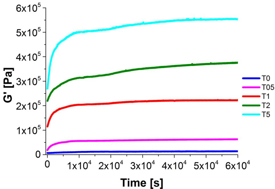
Fig. 5.12 Time evolution of the shear Elasticmodulus  $G'$  for A50C50 blends
