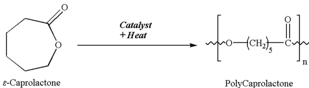
Fig. 3.3 Ring Opening Polymerization scheme for Poly( $\epsilon$ -caprolactone)
