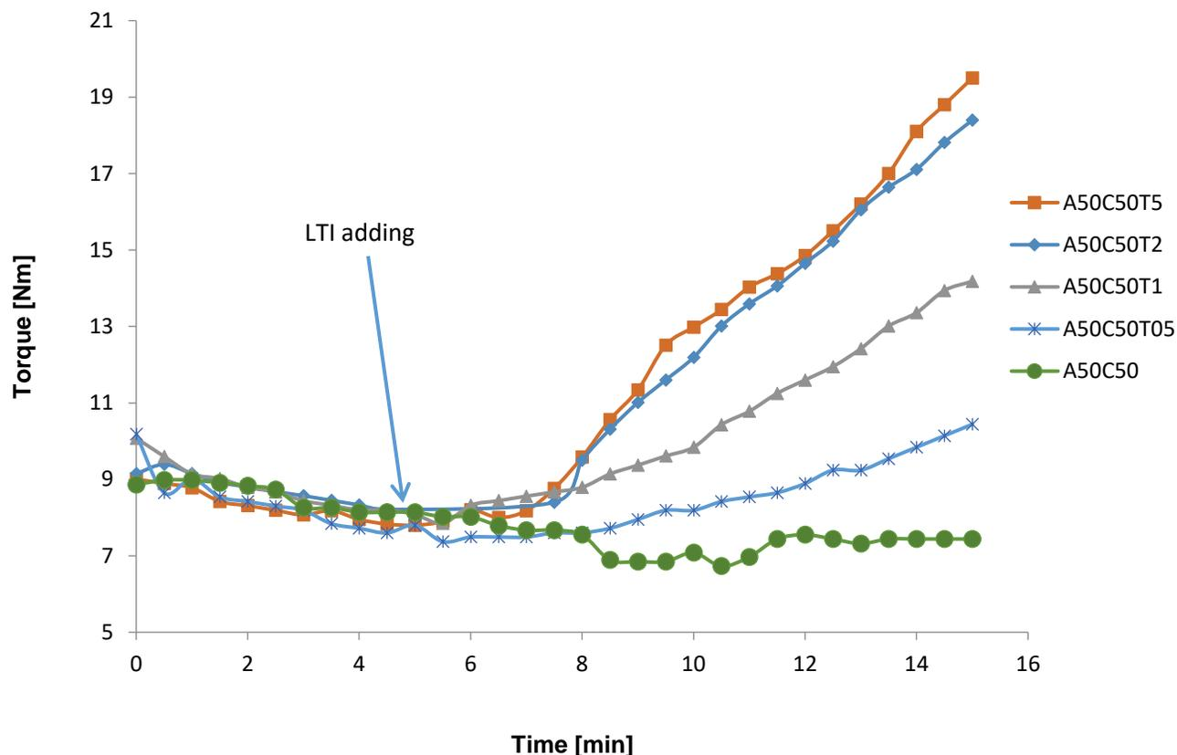
Fig. 5.2 Torque vs Time trends of A50C50 blends with various LTI amounts
