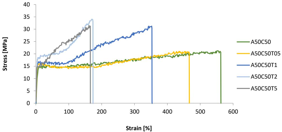
Fig. 5.19, A50C50 extruded physical and reactive blends Stress-Strain trends.
