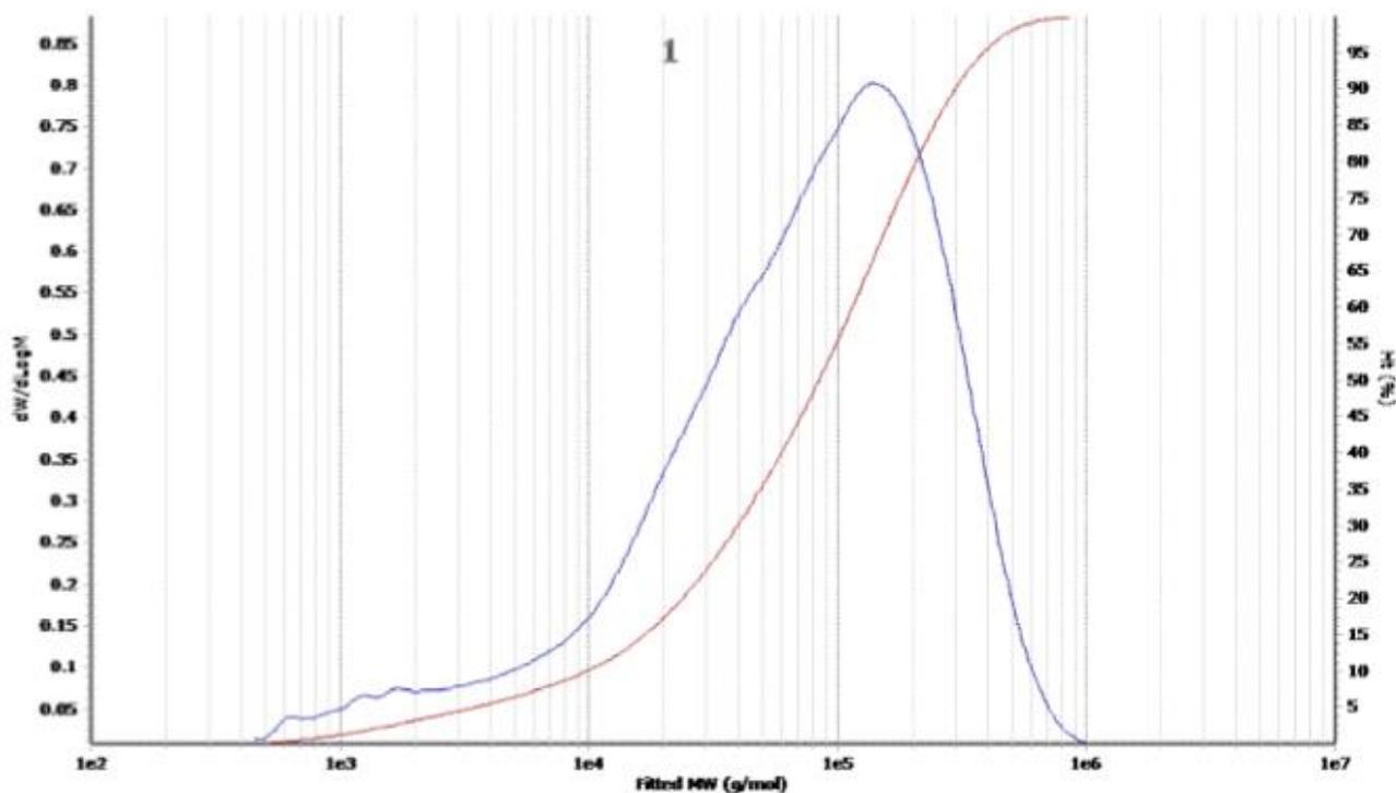
Fig 4.1, Gel Permeation Chromatography data (top PLA, bottom PCL)
