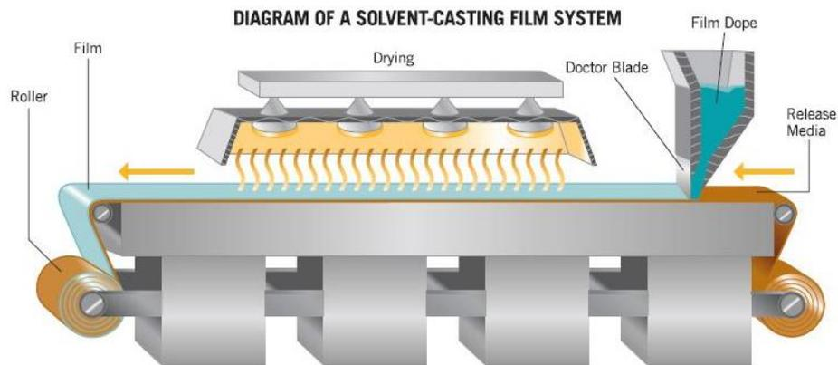
Fig. 2.5 Schematics of Solvent Casting process
