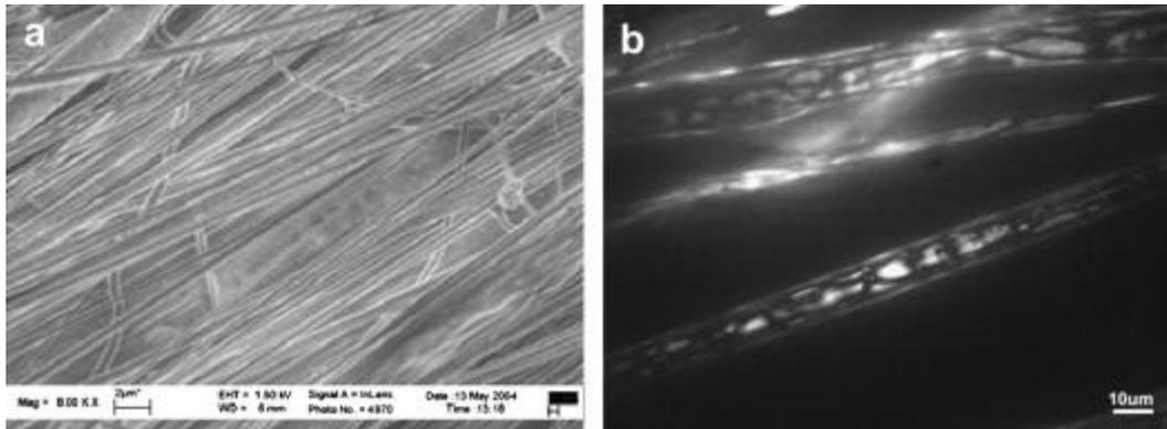
Fig. 1.11 (a) Aligned BSA encapsulated PCLEEP fibres electrospun at 1 mL/h. (b) Fluorescein isothiocyanate-conjugated bovine encapsulated electrospun fibres of PCLEEP. [24]
