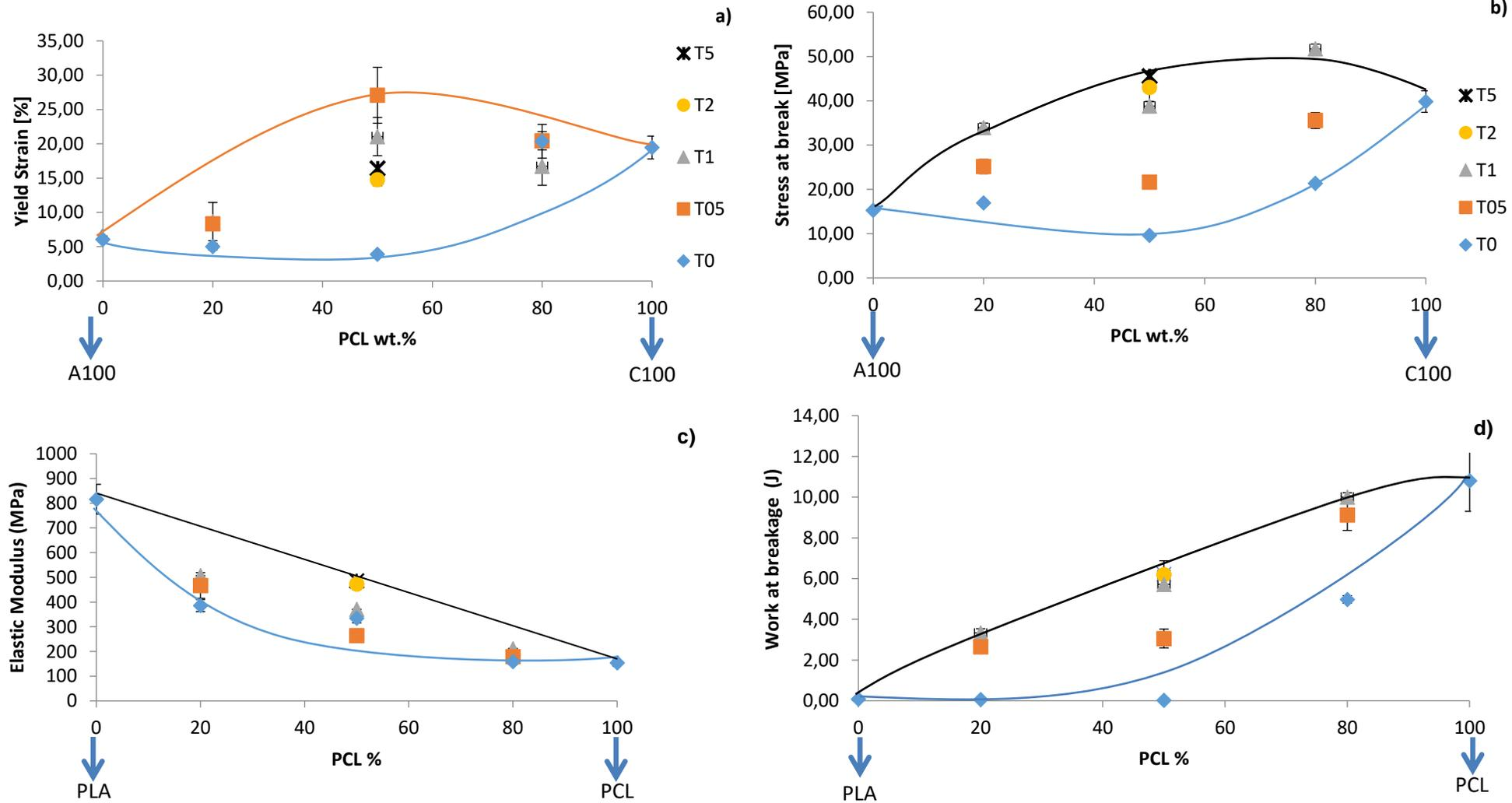
Fig. 5.8 a) Yield Strain, b) Stress at Break, c) Elastic Modulus, d) Work at Breakage of Physical and Reactive Blends by PCL wt%
