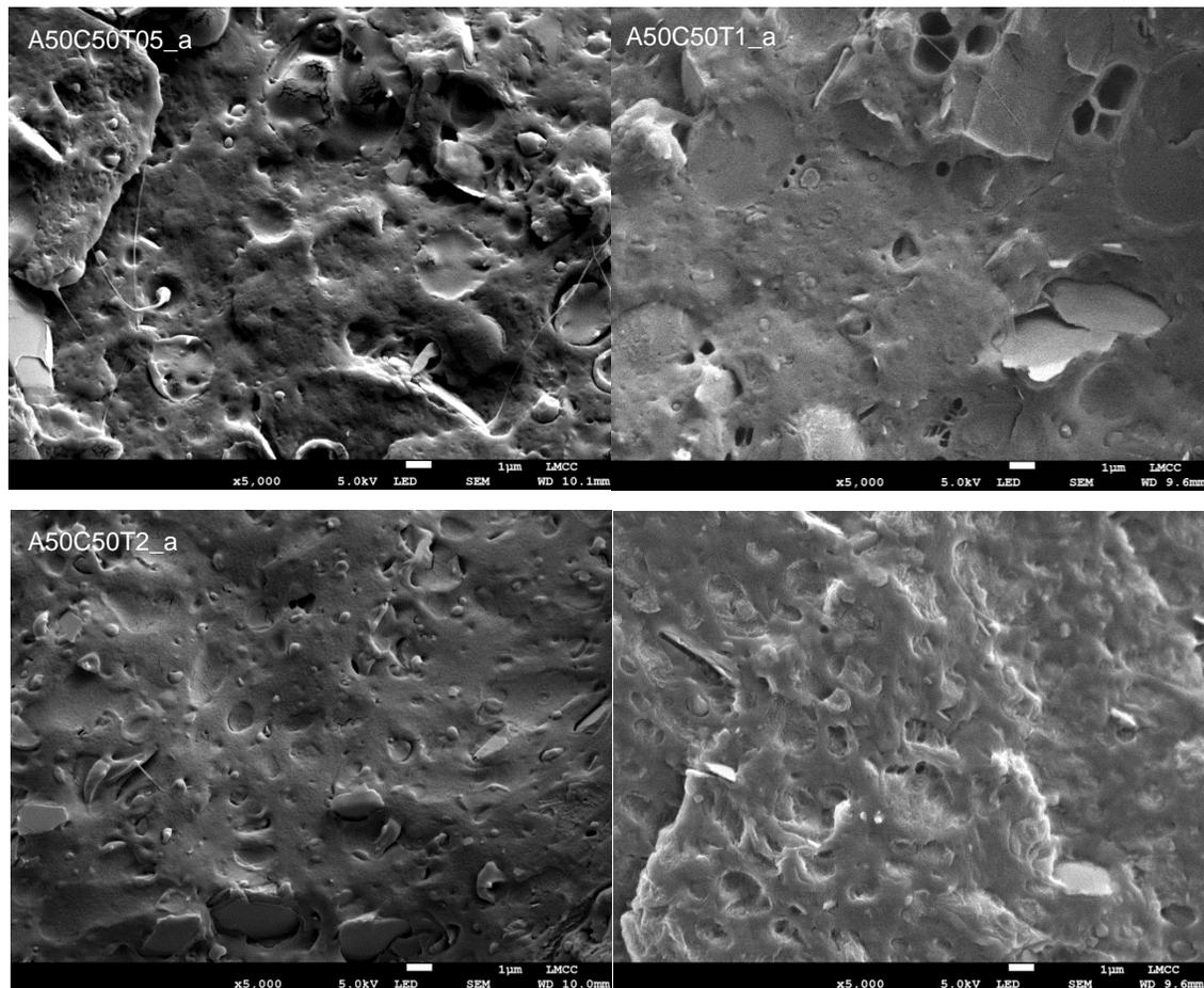
Fig. 5.15 SEM images of reactive blends after rheology tests.
