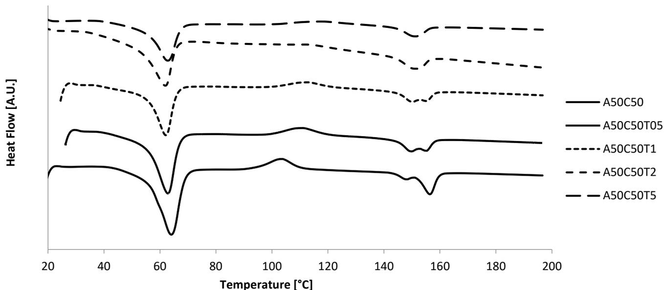
Fig 5.10 A50C50 Physical and Reactive Blends Thermograms, LTI amount effect
