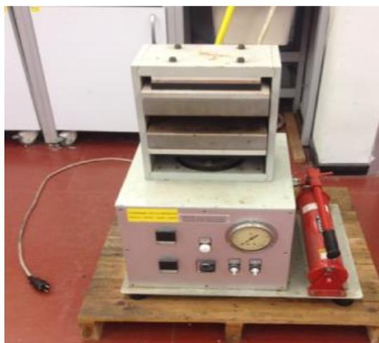
Fig. 4.4 Compression Moulding Press
