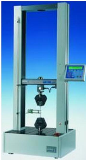
Fig. 4.6 Lloyd LR 10K Universal Testing Machine
