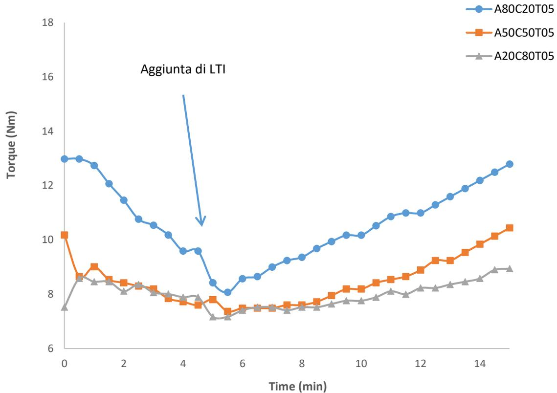
Fig. 5.3 Torque vs Time trends of T05 blends
