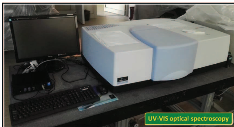
Figure A5: UV-VIS spectrophotometer located in the laboratories of the University of Messina, Italy.
