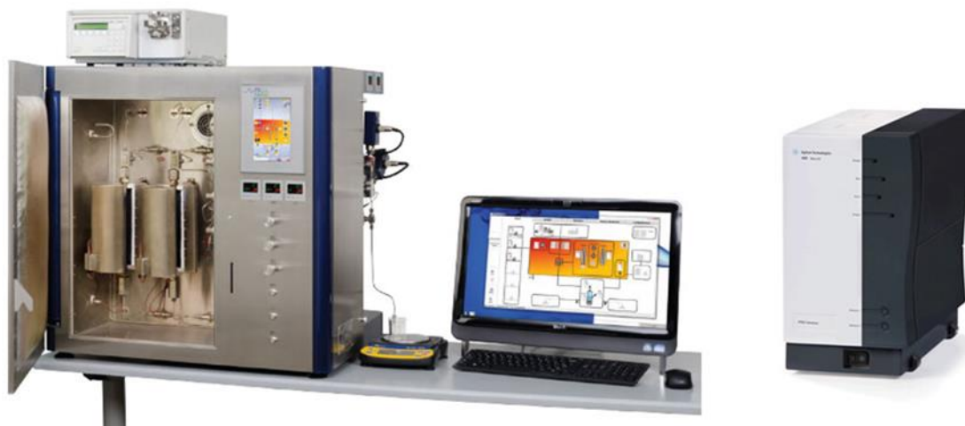
Figure 5.1 Microactivity Efficient equipment (Micromeritics) used for the catalytic CO 2 methanation tests.
