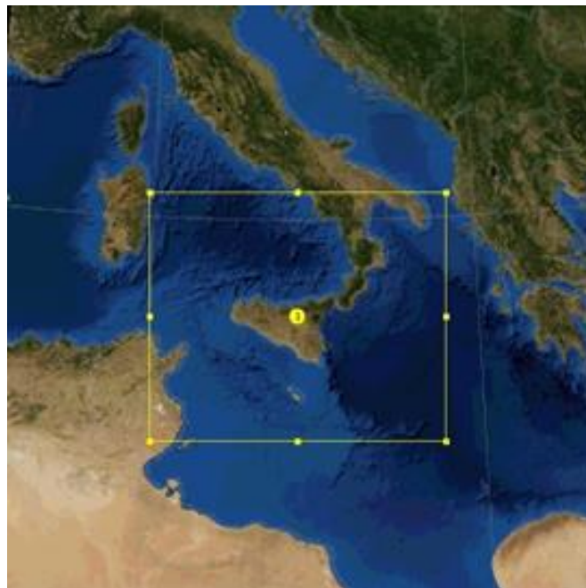
Fig 58. Map of the spatial domain used by the WRF model. The domain is centered on Sicily. The model is configured with horizontal grid spacing of 5km and a time interval resolution of 1h
