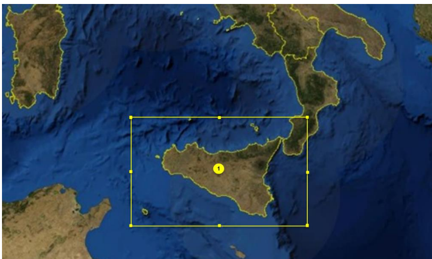
Fig. 42: Map of the spatial domain used by the WRF model. The domain is centered on Sicily. The model is configured with horizontal grid spacing of 5km and a time interval resolution of 1h
