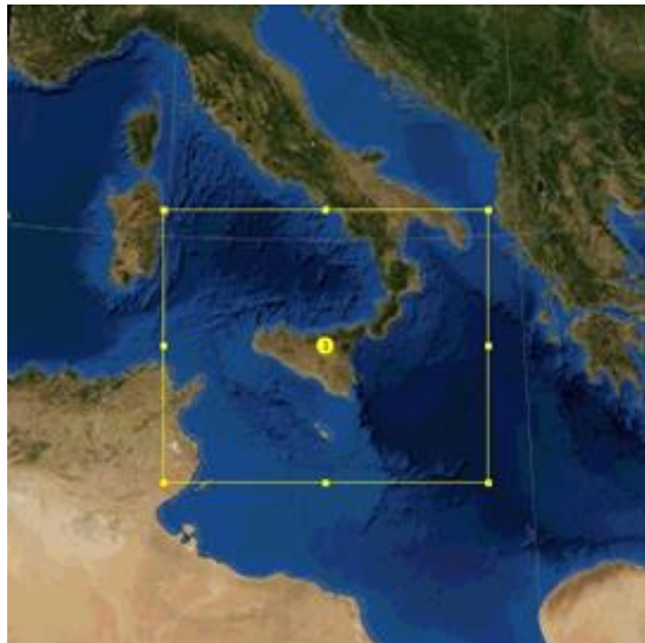
Fig 52. Map of the spatial domain used by the WRF model. The domain is centered on Sicily. The model is configured with horizontal grid spacing of 5km and a time interval resolution of 1h
