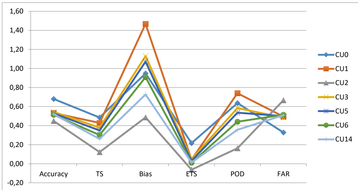
Fig 57: Graphic of indexes calculated for each simulation performed by modifying the physical parameterization of the convective processes of the WRF model. It shows that the CU0 (blue line) is the most reliable and accurate solution. The CU2 (green line) is the worst. CU1 (red line), CU3 (violet line) and CU5 (light blue line) show only small differences and they are the only ones that tend to overestimate the rain. The CU14 and the CU6 (orange line) schemes are only slightly better than the CU2
