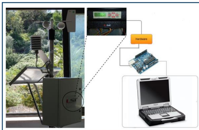
Fig. 8: Weather station-Arduino Monitoring System
